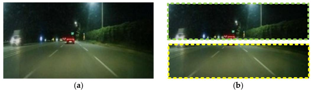
**Figure 5.** Result of ROI: (a) input image; and (b) upper area used for distinguishing between day and night, lower area used for lane detection.
