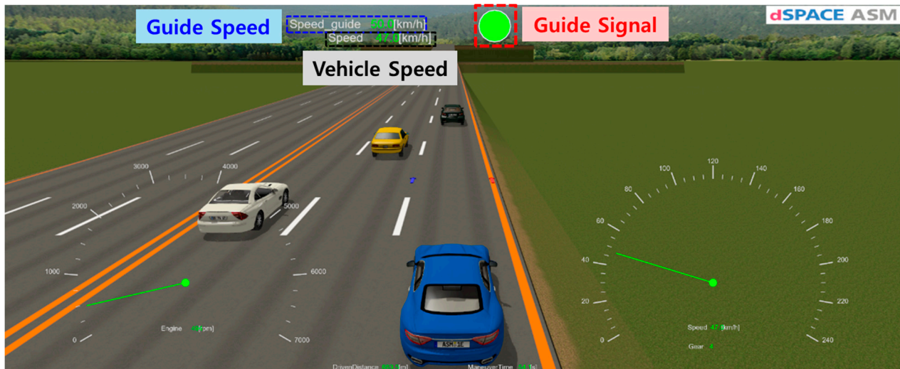
Figure 10. Visual guidance for cooperative eco-driving in the MotionDesk simulation.
