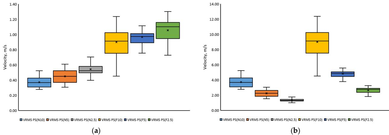
**Figure 9.** Summary of RMS velocity values in the steady motion phase: (a) normal and fast operator hand movements for the tested size ratios and (b) normal and fast effector movements for the tested size ratios.
