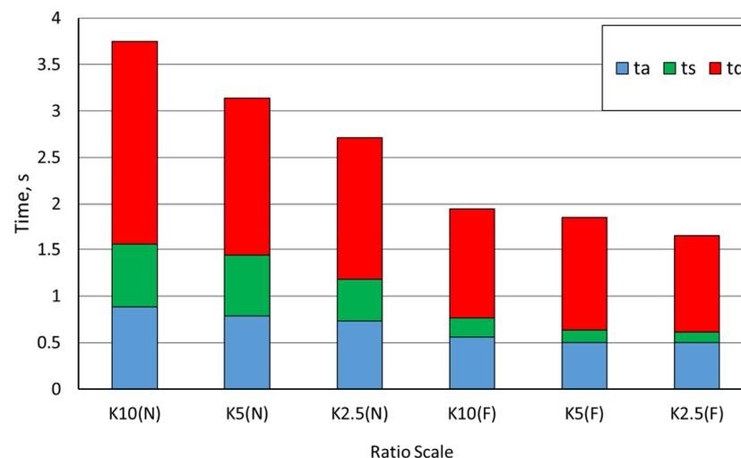
**Figure 8.** Summary of durations  $t_a$ ,  $t_s$ , and  $t_d$  in whole movement; N—normal movement, F—fast movement.
