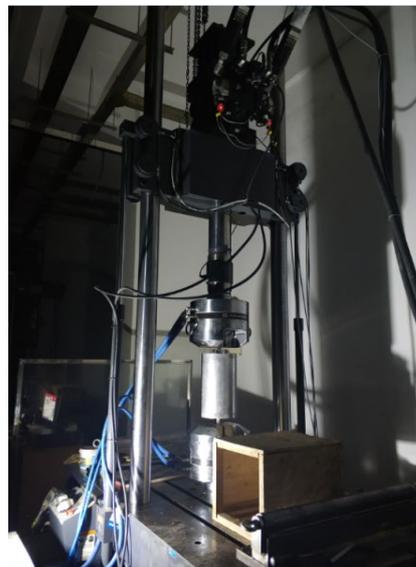
**Figure 10.** Loading schematic of DSCCP shock absorber.
