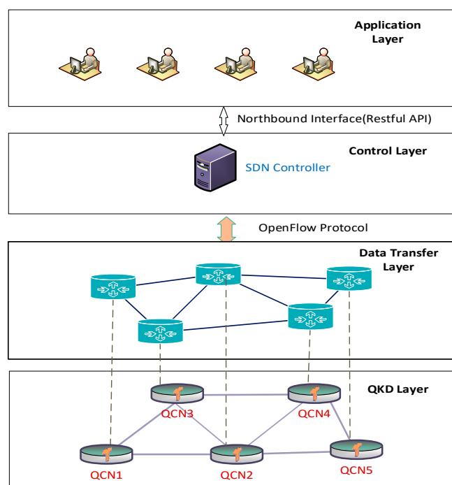
**Figure 1.** SDN-based QKD network architecture.
