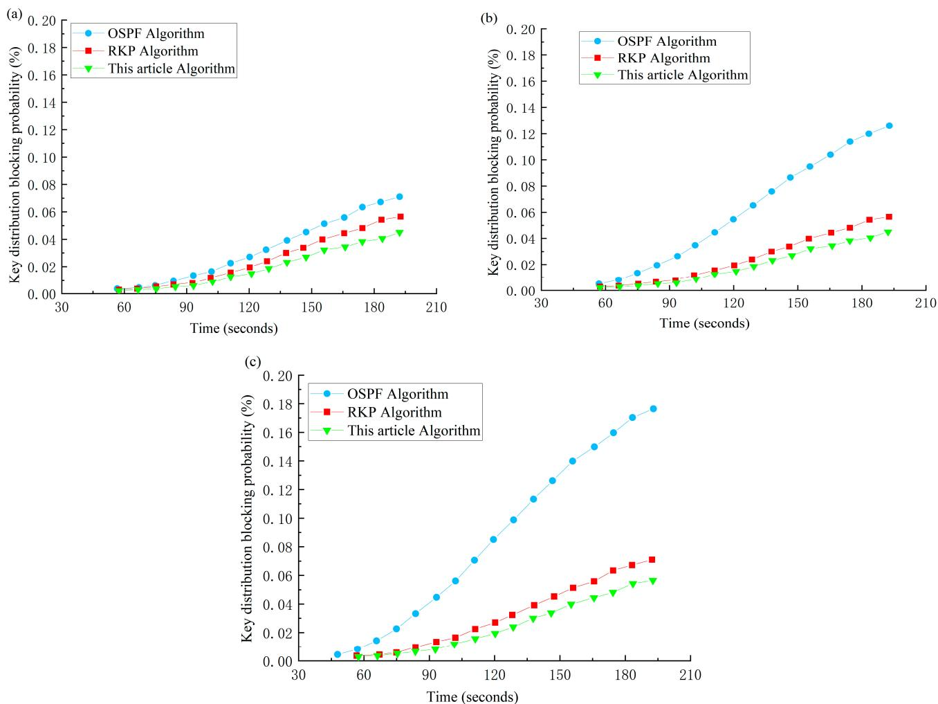
**Figure 8.** (a) Key blocking probability when traffic volume is 50 Erlang; (b) Traffic blocking probability when traffic volume is 100 Erlang; (c) Traffic blocking probability when traffic volume is 200 Erlang.
