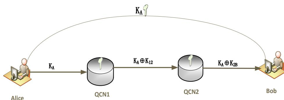
**Figure 2.** Key relay process in QKD network communication based on trustworthy relays.
