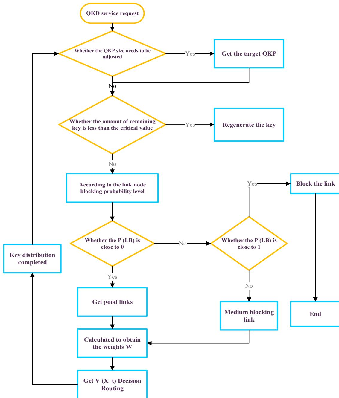
**Figure 5.** Algorithm optimization design flowchart.
