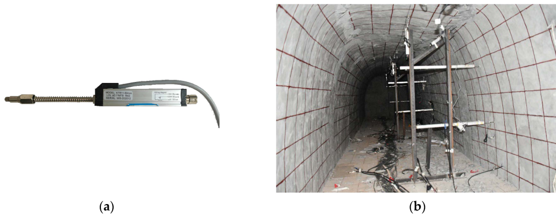
Figure 5. Displacement sensor and bracket: (a) KD2009T displacement sensor and (b) displacement sensor bracket.
