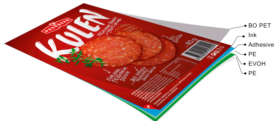
Figure 1. Layout of Kulen flexible packaging with an overview of individual material layers.
