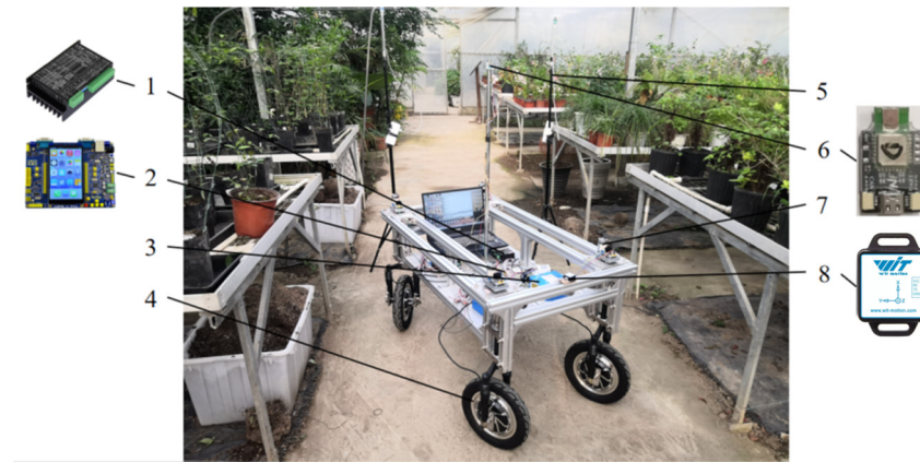
Figure 1. Test prototype and test environment. 1. Motor driver, 2. Microcontroller, 3. Lithium battery, 4. Wheel motor, 5. UWB base station, 6. Mobile tag, 7. Servo, 8. Electronic gyroscope.
