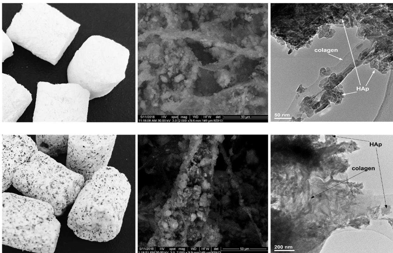
**Figure 11.** Experimental composite materials for bone substitutes type collagen–hydroxyapatite (first line) and collagen–hydroxyapatite–magnesium (second line): left row (up and bottom) macroscopic view, middle row (up and bottom) scanning electron microscopy image, right row (up and bottom) transmission electron microscopy image [99].
