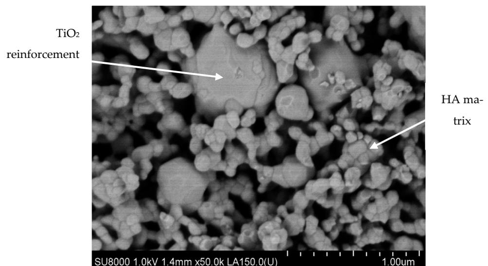
**Figure 7.** SEM micrograph of HA/ $\text{TiO}_2$  biocomposite processed by TSS technology (Courtesy of Prof. Oana Gingu, University of Craiova, Faculty of Mechanics).
