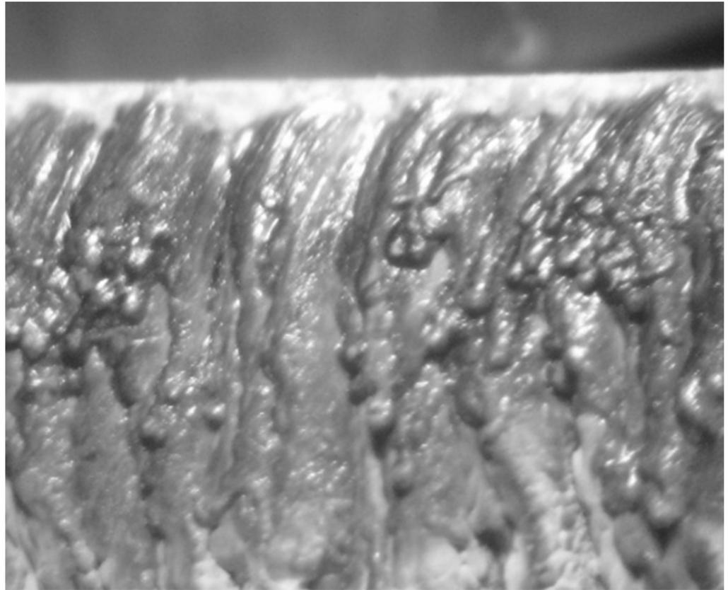
**Figure 9.** Macroscopic aspect ( $\times 8$  magnification) of HAP/TiO<sub>2</sub> biocomposites after laser micro-machining at 280 V, 60 Hz and 0.35 ms as pulse duration. The average obtained roughness  $R_a = 15.4 \mu\text{m}$  [94].
