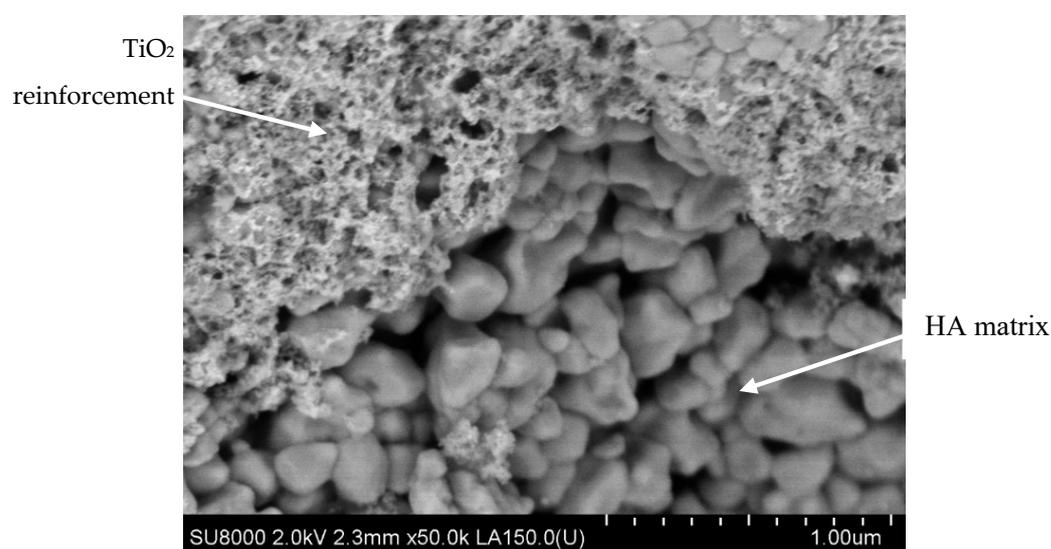
**Figure 8.** SEM micrograph of HA/ $\text{TiO}_2$  biocomposite processed by SPS technology (Courtesy of Prof. Oana Gingu, University of Craiova, Faculty of Mechanics).
