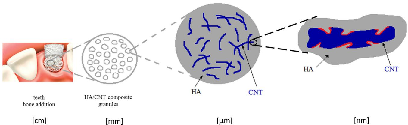
**Figure 6.** Schematic representation of the micromechanical interlock model of the interface between the HA and CNTs, providing a physical bonding at the interface level (red curves).
