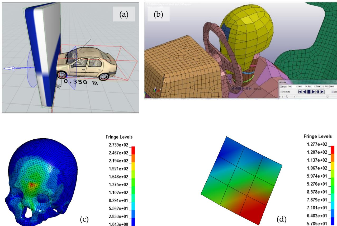
**Figure 13.** FEM simulation of (a) one sedan frontal impact with (b) the “pilot” having an alloplastic bone graft in frontal-cranial position; (c) von-Mises stress map for the skull and (d) von-Mises stress map for the graft (Courtesy of Prof. Oana Gingu, University of Craiova, Faculty of Mechanics).
