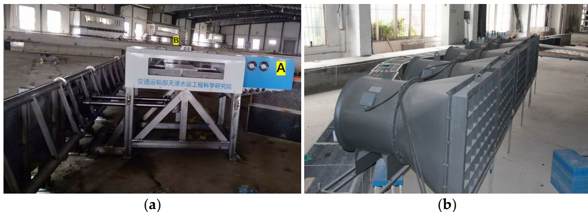
Figure 5. Facilities for wave and wind simulations. (a) Wavemaker. (b) Fan array for wind. (In the subfigure a, the servo motor part is marked by letter A and the fixed support part is marked by letter B).
