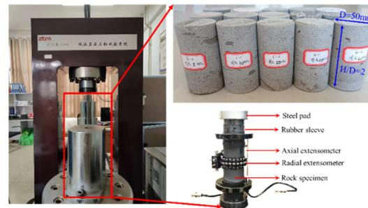
Figure 1. Sandstone specimens and test system.
