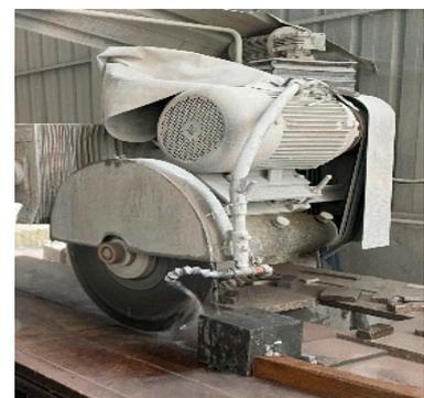
(b) Specimen cutting instrument
