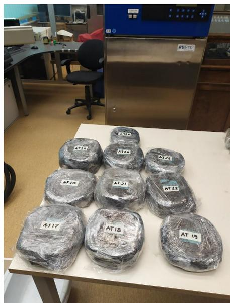
**Figure 6.** Preparation of specimens for the oedometer tests.
