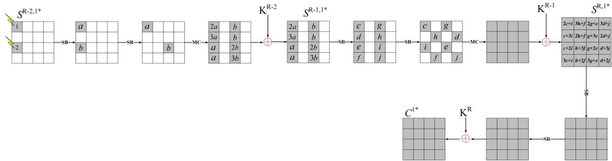
Figure 7. The propagation of the Dcor fault induced at  $S_1^{R-2}$  and  $S_9^{R-2}$ .
