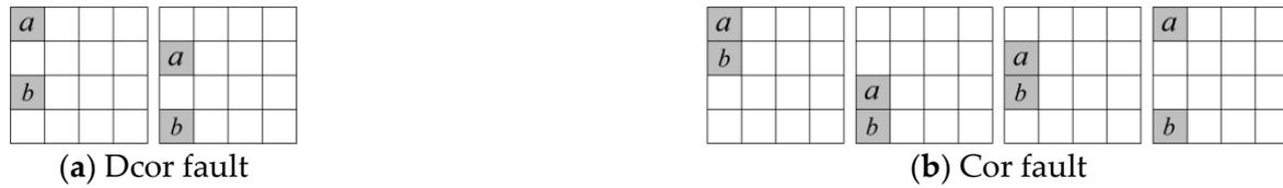
Figure 6. The Dcor and Cor fault model. (a) Two-byte faults induced at the first column with discontinuous rows; (b) two-byte faults induced at the first column with contiguous rows.
