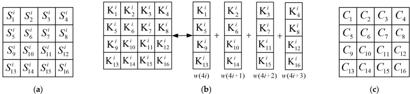
**Figure 1.** Use of a  $4 \times 4$  matrix to represent the state, the key, and the ciphertext. (a) The state; (b) the key; (c) the ciphertext.
