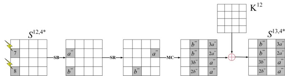
Figure 12. The propagation of faults ‘7’ and ‘8’ induced at  $S_5^{12}$  and  $S_{13}^{12}$ .
