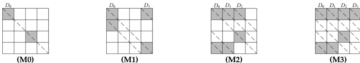
**Figure 5.** The example of fault models. (M0) The random fault is induced in one of the diagonals; (M1) a random non-zero fault occurs at most across two diagonals; (M2) a random non-zero fault occurs at most across three diagonals; (M3) a random non-zero fault occurs at most across four diagonals.
