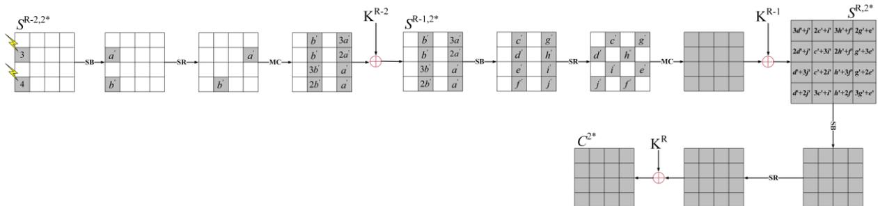
Figure 8. The propagation of the Dcor fault induced at  $S_5^{R-2}$  and  $S_{13}^{R-2}$ .
