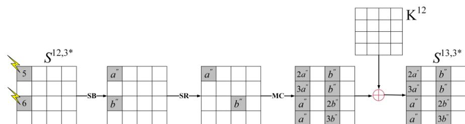
Figure 11. The propagation of faults '7' and '8' induced at  $S_1^{12}$  and  $S_9^{12}$ .
