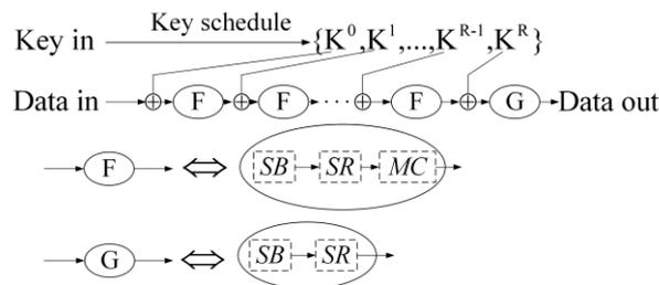
Figure 2. The encryption process of AES.
