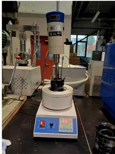
**Figure 1.** Mixing of asphalt mastics.
