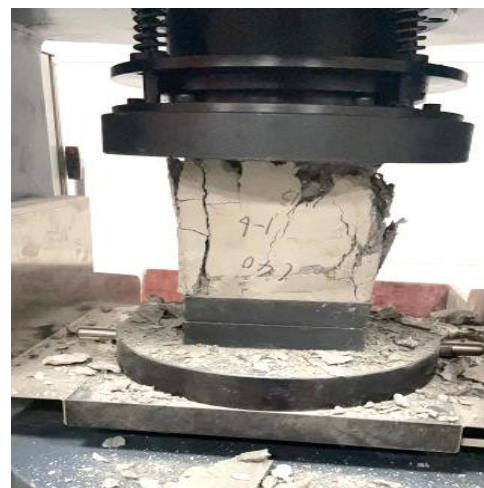
Figure 4. Testing process of concrete.
