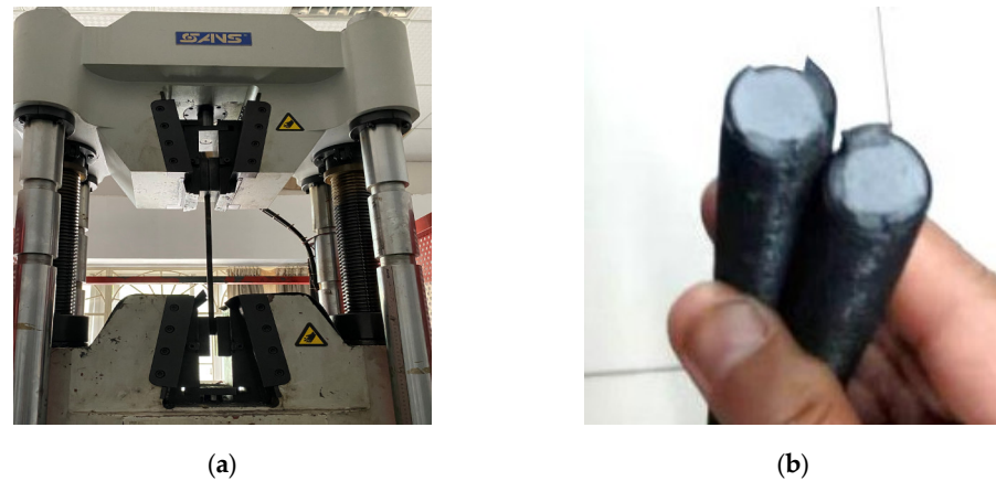
Figure 5. Bond Strength test. (a) Loading setup. (b) Broken section of bolt.
