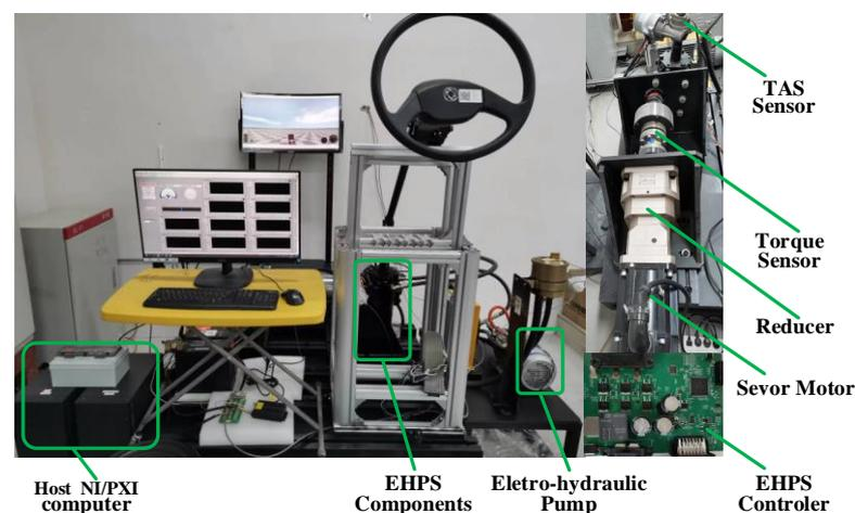
Figure 9. Structure of hardware-in-the-loop test bench.
