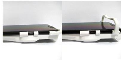
**Figure 11.** Slider cover of Prototype 3 at 0 and 90 degrees.
