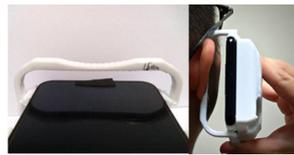
**Figure 14.** Curve-shaped slider cover of Prototype 3.
