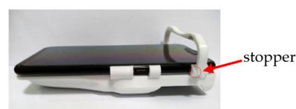
**Figure 12.** Stopper is added to the slider cover of Prototype 3.
