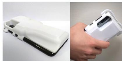
**Figure 18.** Curved handle of Prototype 3.
