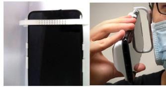
**Figure 13.** Small holes are added in Prototype 3.
