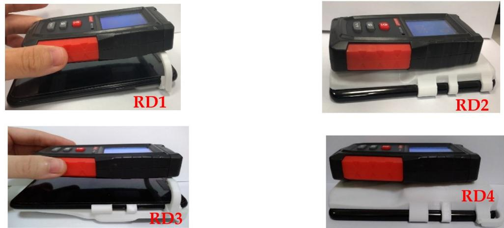
Figure 20. Experiment with measuring phone radiation when the phone is used with RD1 to RD4.
