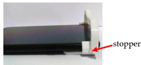
**Figure 2.** Stopper is added to the slider cover of Prototype 1.
