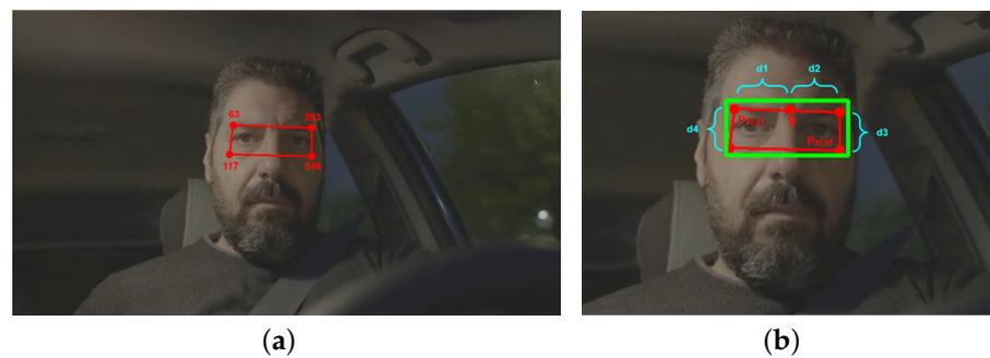
**Figure 2.** ROI correction. (a) ROI with the 4 points. (b) ROI correction method.
