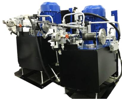
**Figure 1.** Two identical hydraulic system durability test rigs with wear particles (right, front) and test dust (MTD) (left, rear).
