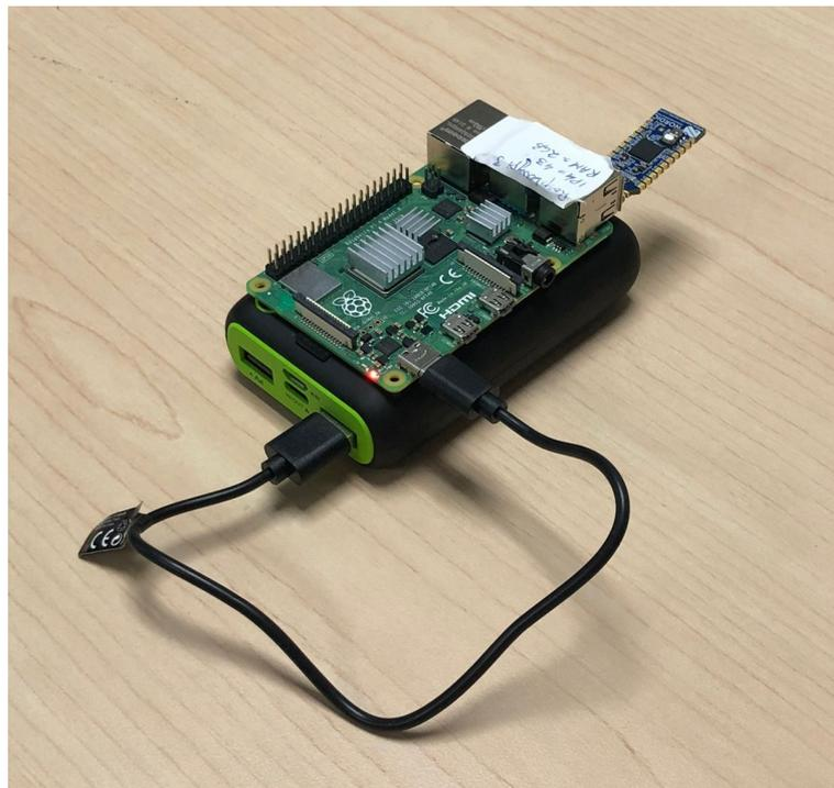
**Figure 3.** Thread node based on Raspberry Pi 4B, Nordic nRF52840 dongle, powered by a power bank.
