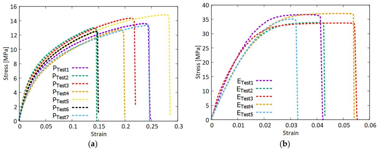
**Figure 6.** Adhesives tensile tests: (a) polyurethane (ADEKIT A 236/H 6236); (b) Epoxy (SIKAPOWER-1277).
