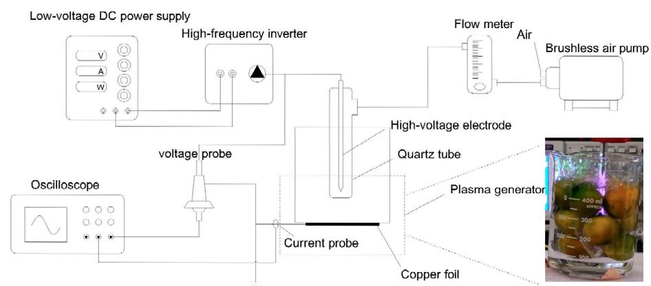
**Figure 1.** Plasma generation device diagram.
