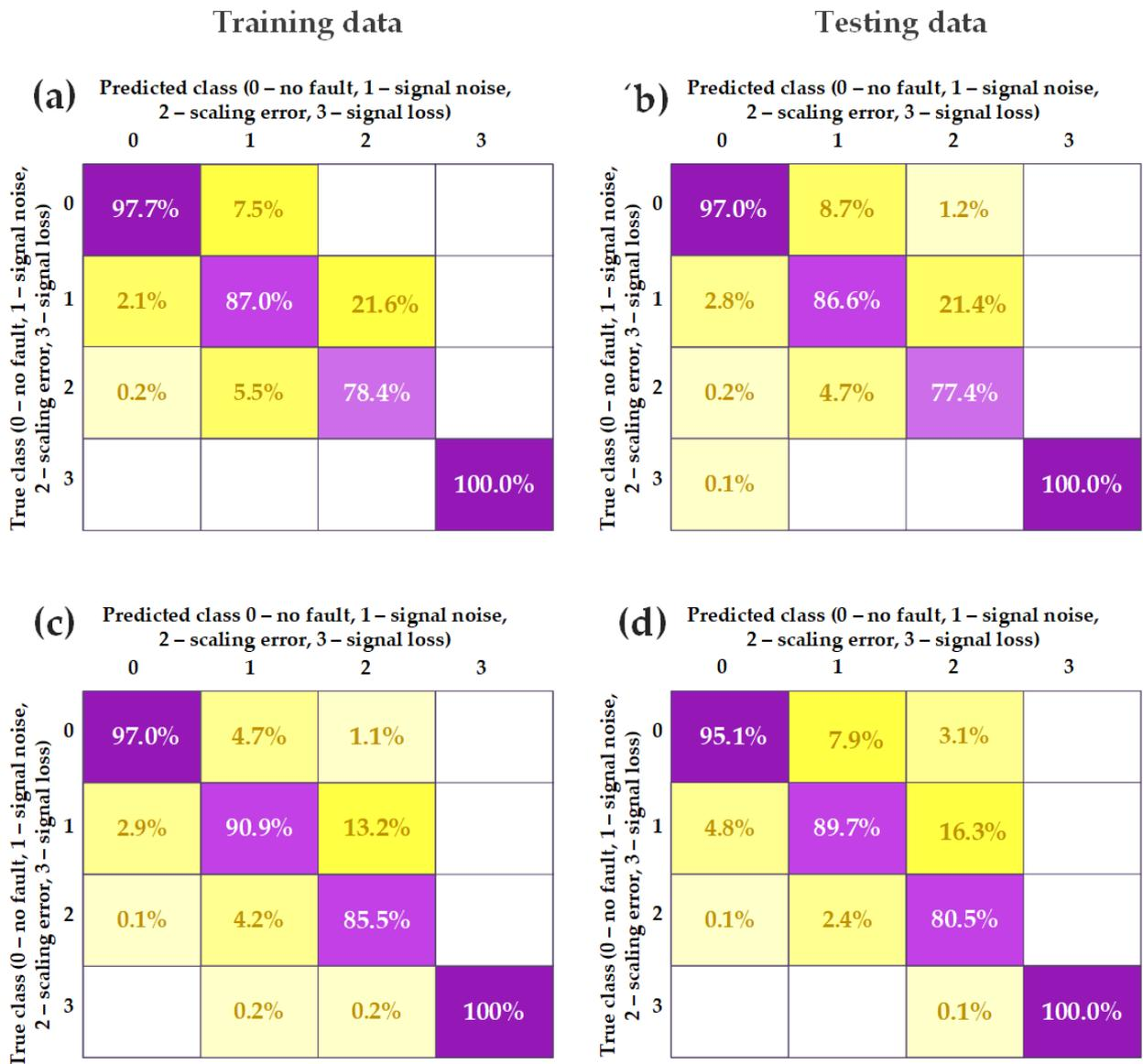
Figure 11. Confusion matrixes with effectiveness obtained by MRAS-based classifier for training (a) and testing data (b) and SMO-based classifier for training (c) and testing data (d).
