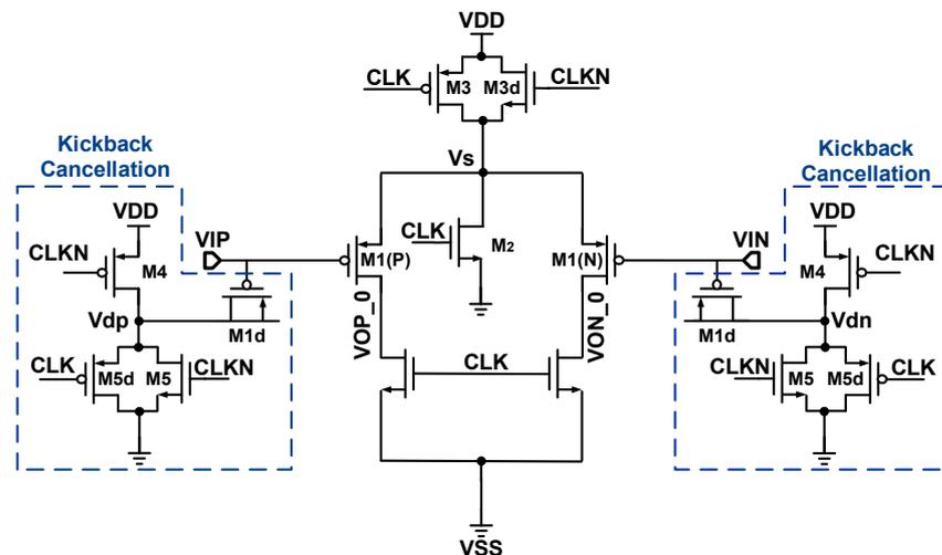
Figure 9. The preamplifier stage of the comparator.
