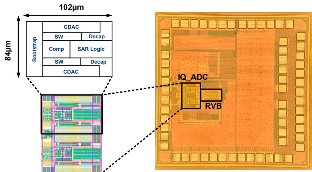
Figure 17. Chip micrograph and layout zoomed-in view of the SAR ADC core.
