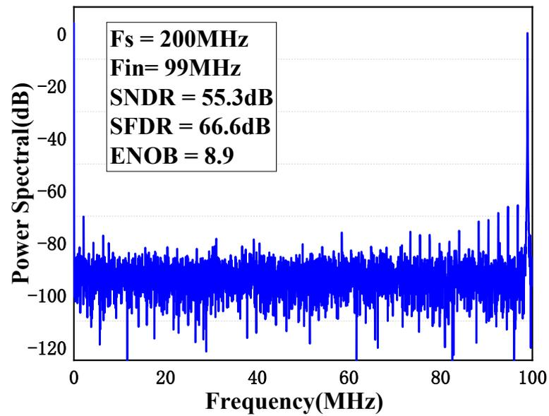
Figure 19. FFT plot with a 99 MHz input frequency at 200 MS/s.
