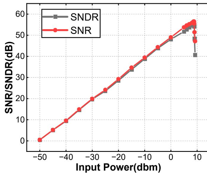
Figure 21. Measured performance versus input power.
