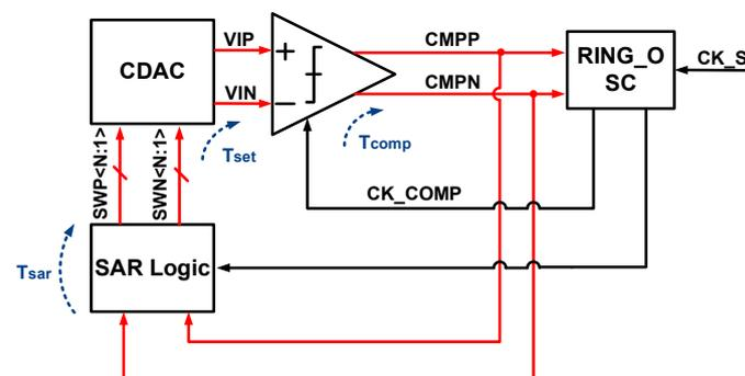
Figure 6. Data path during the SA phase.
