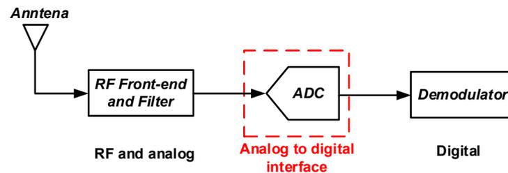
Figure 1. The role of ADC in the receiver.
