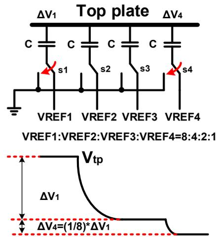
Figure 4. Voltage jumping during the 4-reference voltage scheme.
