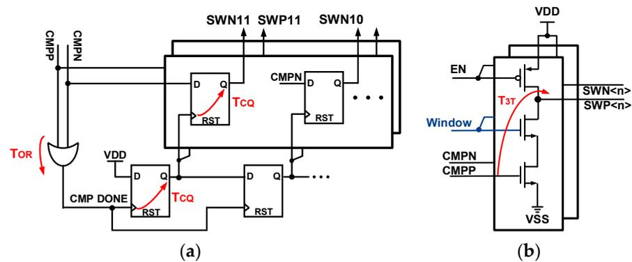
Figure 13. (a) Critical path of traditional SAR logic; (b) critical path of the 3-T cell.
