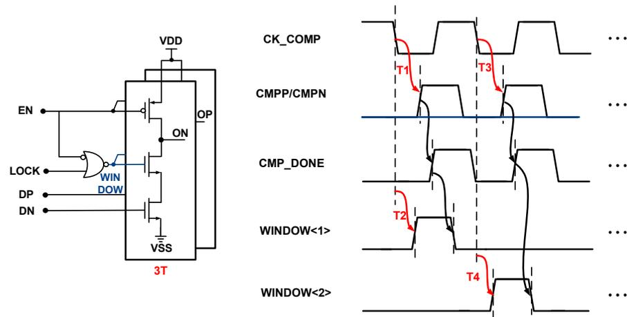
Figure 15. The proposed tri-state gate and corresponding timing diagram of the window-opening strategy.
