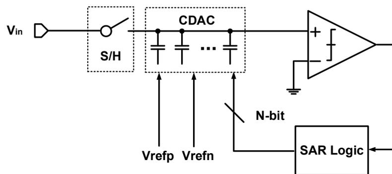
Figure 2. Architecture of a conventional SAR ADC.
