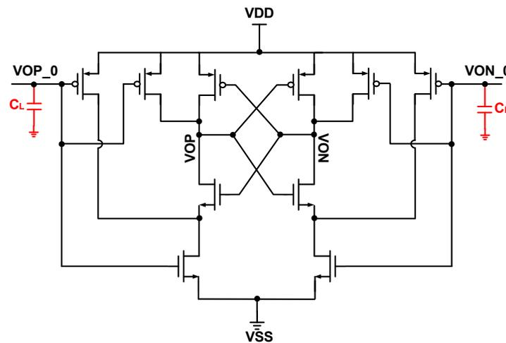
Figure 10. The latch stage of the comparator.
