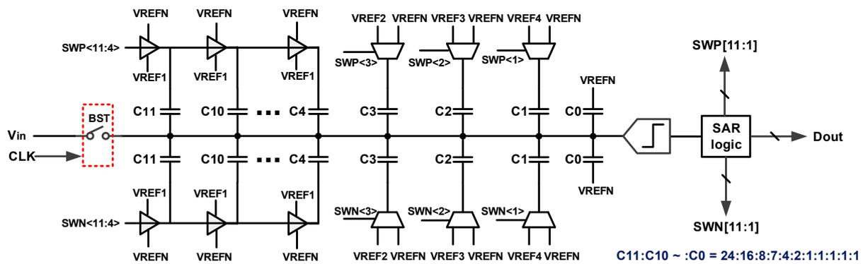
Figure 3. Architecture of the proposed SAR ADC.
