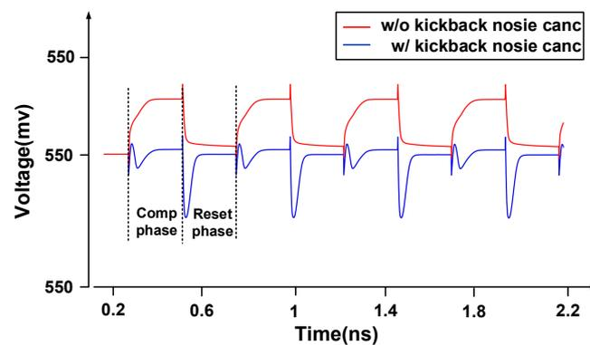
Figure 12. The comparator input voltage with/without a kickback cancellation circuit.
