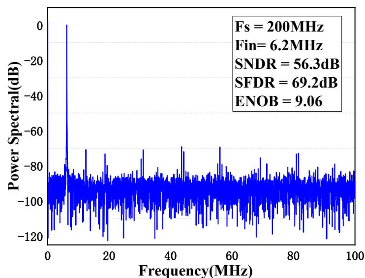
Figure 18. FFT plot with a 6 MHz input frequency at 200 MS/s.
