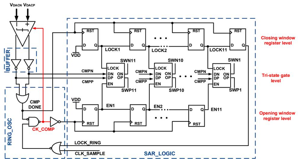
Figure 14. The proposed SAR Logic.
