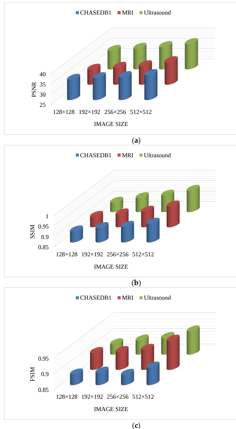
Figure 11. Performance of proposed HCPSO-based GDB filter for varying input image sizes in terms of (a) PSNR, (b) SSIM, and (c) FSIM.
