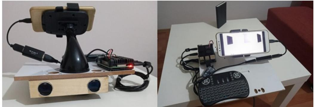
Figure 2. The stereo vision mechanism used in the study.
