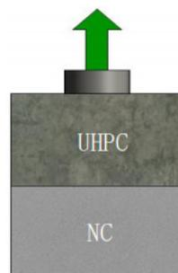
**Figure 2.** Schematic of the pull-off test.
