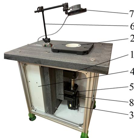
**Figure 14.** Laboratory setup for studying the MM: 1—inductor with PM; 2—working chamber; 3—driving engine; 4—supervision system; 5—support arrangements of the supporting and rotating device; 6—tripod; 7—illumination lamp; 8—bed plate.
