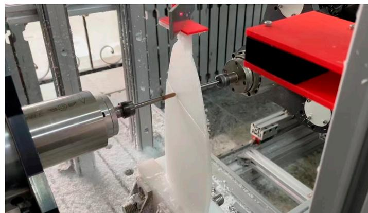
**Figure 9.** The double-sided collaborative machining process of propeller blades.
