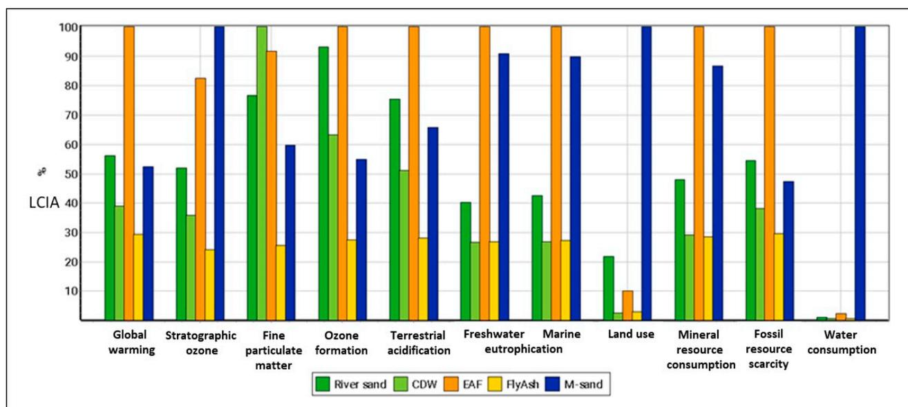
**Figure 2.** Life-cycle impact analysis for subbase layers made from river sand, CDW, EAF, FA, or m-sand (normal scenario).
