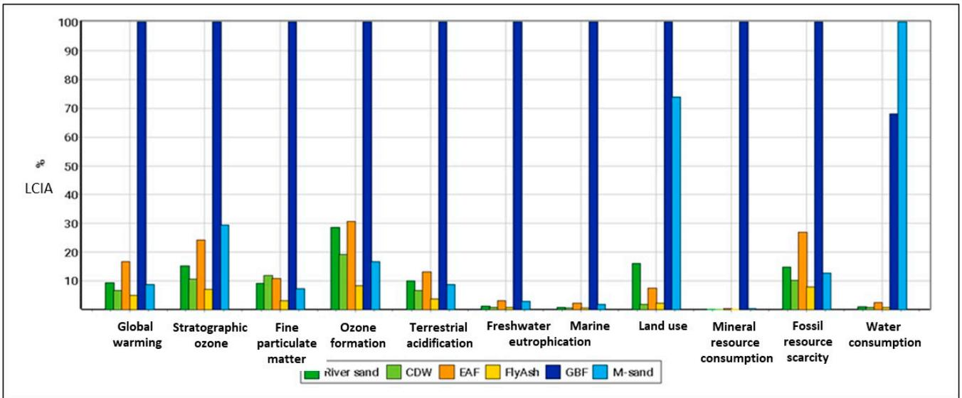
Figure 3. Life-cycle impact analysis for subbase layers made from river sand, CDW, GBF, FA, or m-sand (normal scenario).
