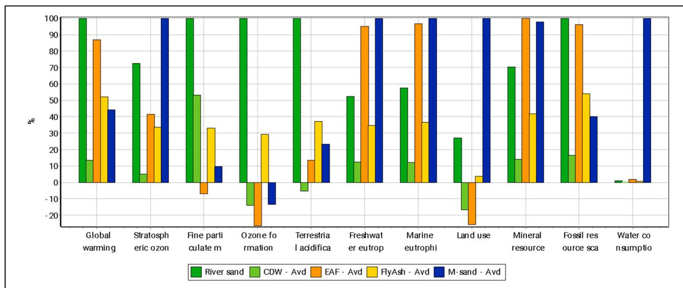
**Figure 6.** Life-cycle impact analysis for subbase layers made from river sand, CDW, EAF, FA, or m-sand (avoidance scenario).
