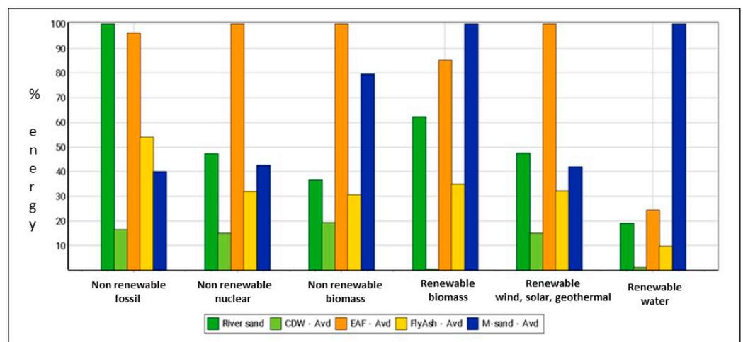
**Figure 8.** Energy demand analysis for subbase layers made from river sand, CDW, EAF, FA, or m-sand (avoidance scenario).
