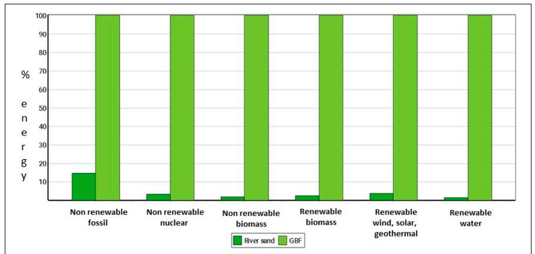
Figure 5. Energy demand analysis for subbase layers made from river sand or GBF (normal scenario).
