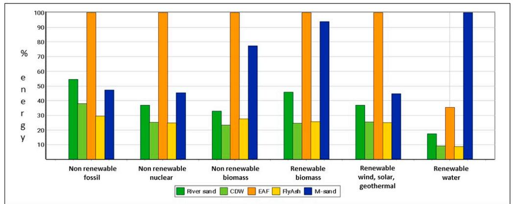
Figure 4. Energy demand analysis for subbase layers made from river sand, CDW, EAF, FA, or m-sand (normal scenario).
