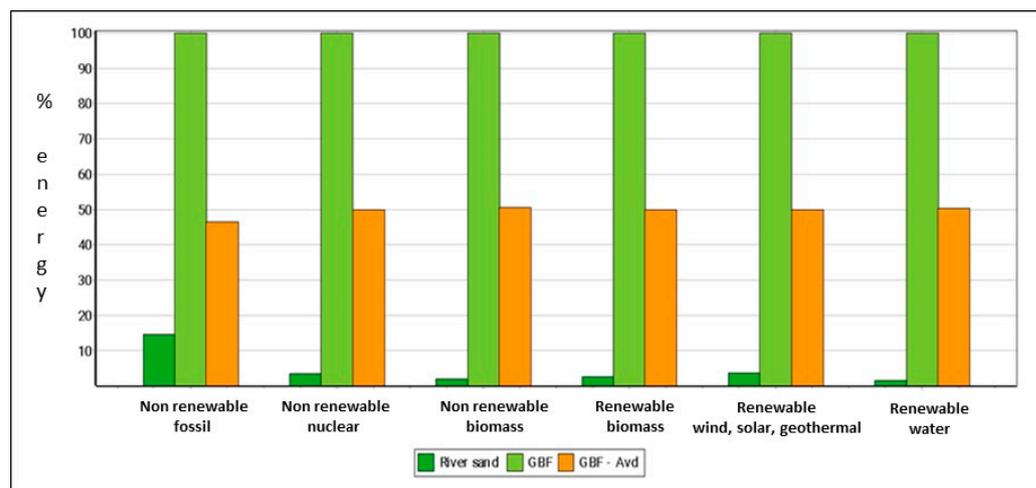
**Figure 9.** Energy demand analysis for subbase layers made from river sand or GBF (avoidance scenario).
