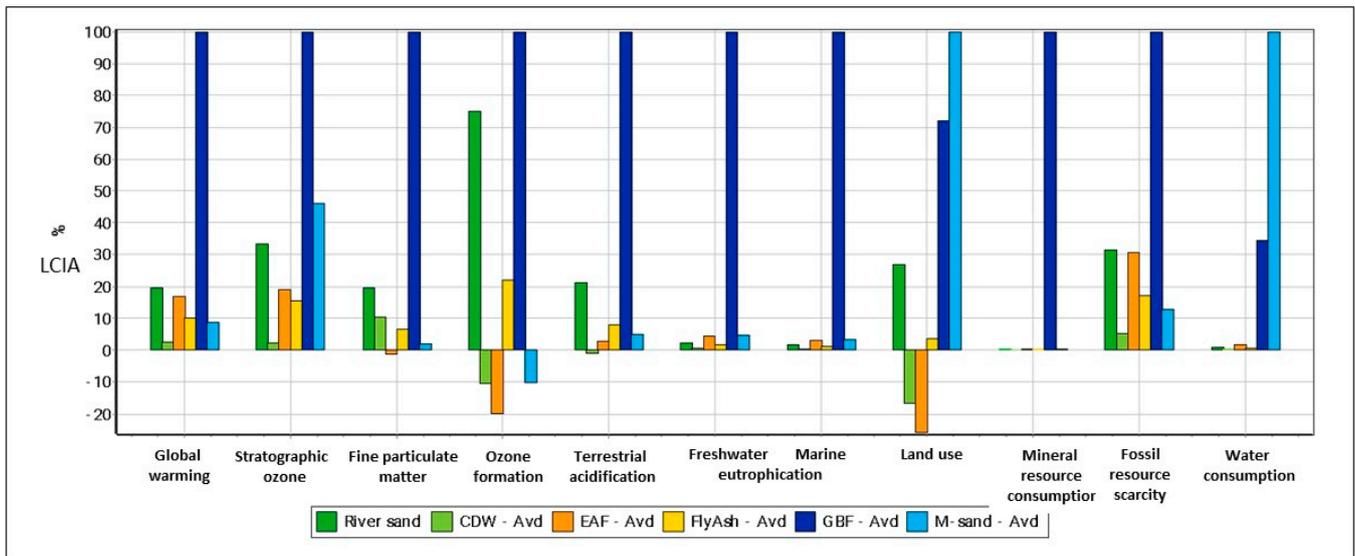
**Figure 7.** Life-cycle impact analysis for subbase layers made from river sand, CDW, EAF, FA, GBF, or m-sand (avoidance scenario).
