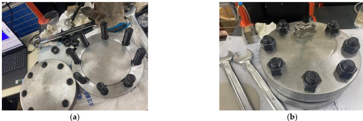
**Figure 1.** Flange fastening device: (a) disassembled, (b) assembled.
