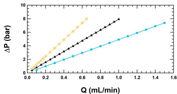
**Figure 6.** Pressure drop as a function of flow rate for the laminar flow of water through the soda glass micro tube (light blue circle), stainless steel microtube (black triangles) and PEEK Beige microtube (beige diamonds).
