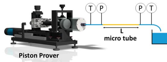
**Figure 1.** Schematic setup of the pipe viscometer with temperature (T) and pressure (P) sensors upstream and downstream of the microtube.
