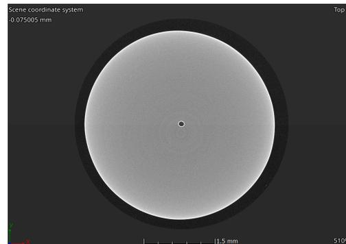
**Figure 3.** Cross-section of the glass microtube determined by means of  $\mu$ -CT method.
