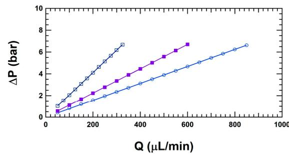
**Figure 7.** Pressure drop as a function of flowrate flow through the glassmicro tube of reference liquid 2AW (blue open circles), reference liquid 2BW (violet solid squares) and reference liquid 5AW (dark blue open squares) with the corresponding linear fit with forced zero intercept.
