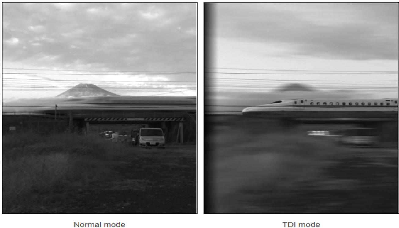
Figure 6. Impact of TDI incorporation in CMOS and CCD sensors [5].
