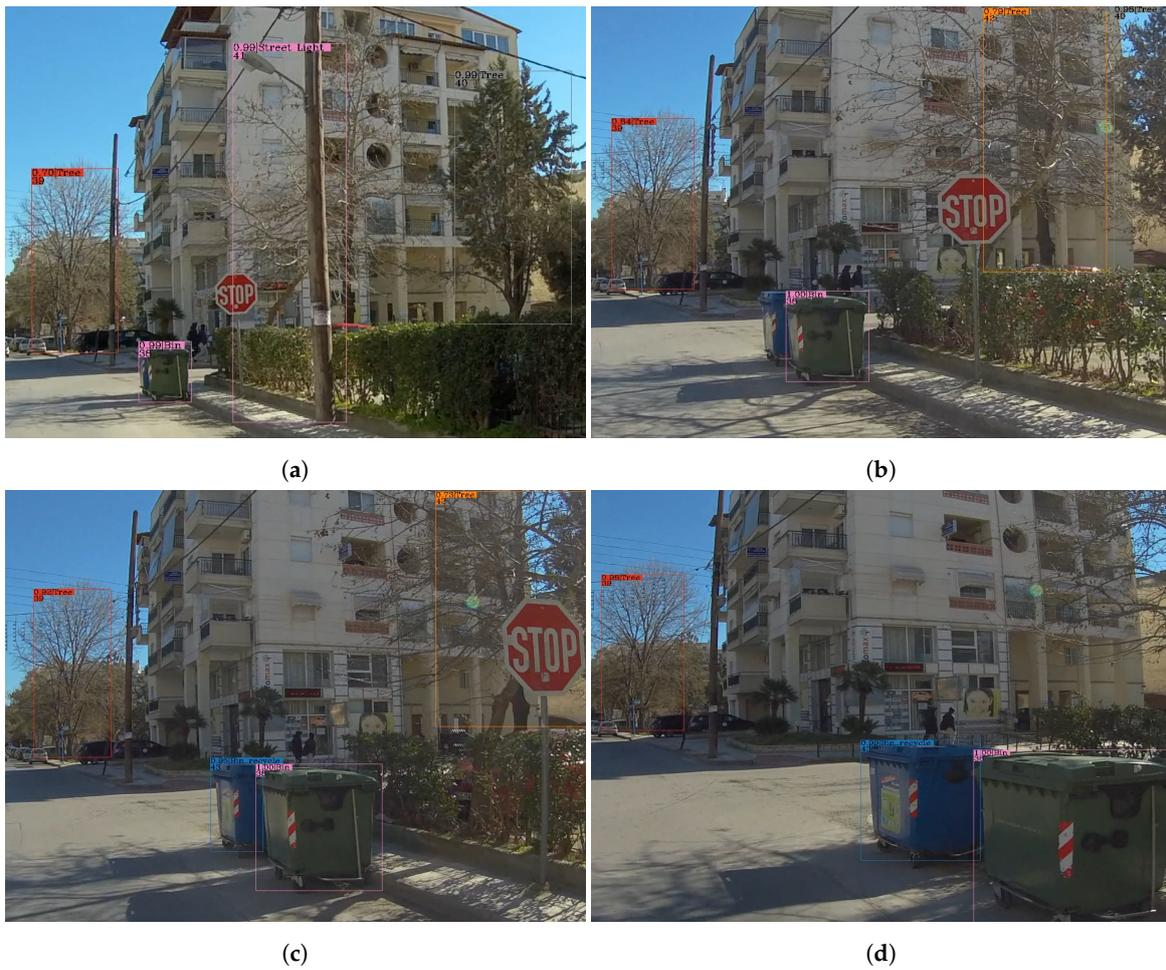
**Figure 6.** Example of object tracking in consecutive frames with the ByteTrack method [41]. (a) First frame. (b) Second frame. (c) Third frame. (d) Fourth frame.
