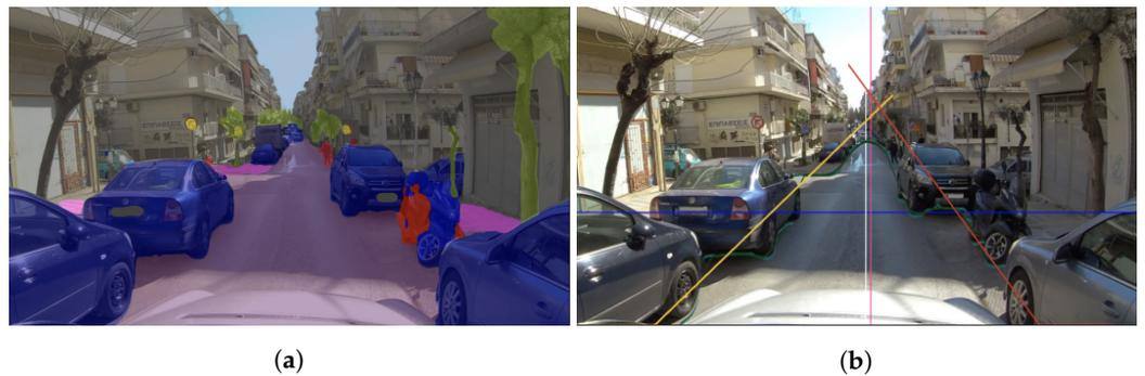
**Figure 3.** Example of object position estimation pipeline. (a) Semantic segmentation with *DeepLabv3+* pre-trained in the *cityscapes* dataset. (b) Road width estimation.
