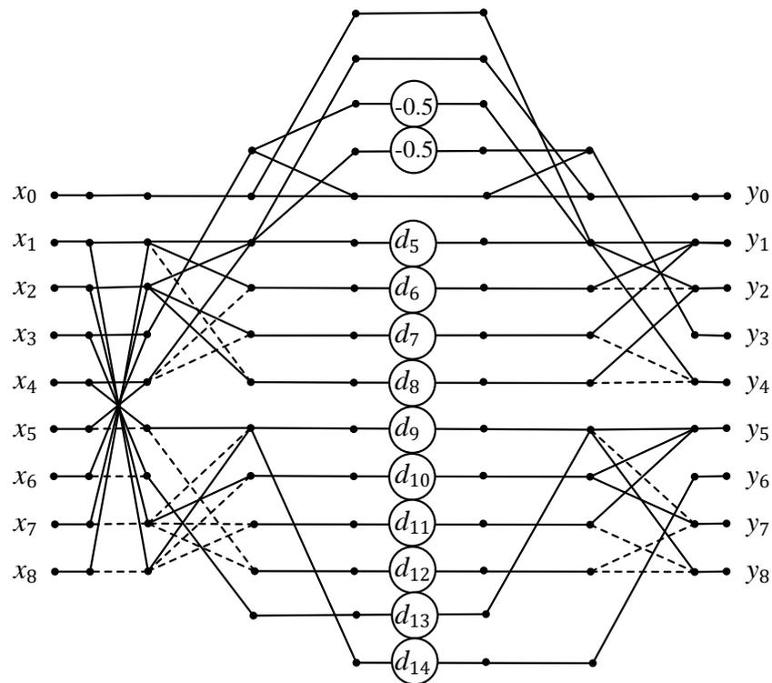
Figure 7. Data-flow diagram of the RDFT algorithm for  $N = 9$ .
