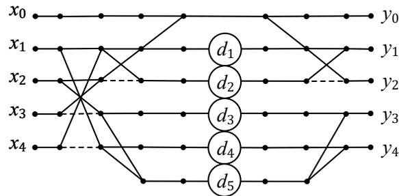
Figure 3. Data-flow diagram of the RDFT algorithm for  $N = 5$ .
