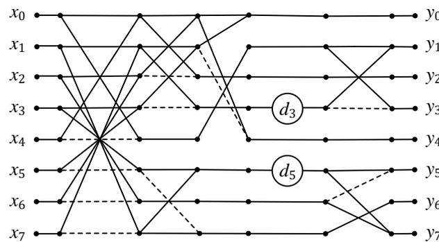
Figure 6. Data flow diagram of the RDFT algorithm for  $N = 8$ .
