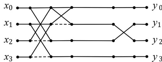
Figure 2. Data-flow diagram of the RDFT algorithm for  $N = 4$ .
