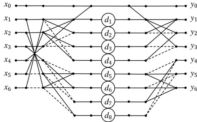
Figure 5. Data-flow diagram of the RDFT algorithm for  $N = 7$ .
