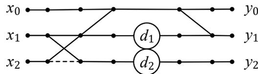
Figure 1. Data-flow diagram of the RDFT algorithm for  $N = 3$ .
