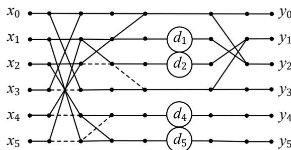
Figure 4. Data flow diagram of the RDFT algorithm for  $N = 6$ .
