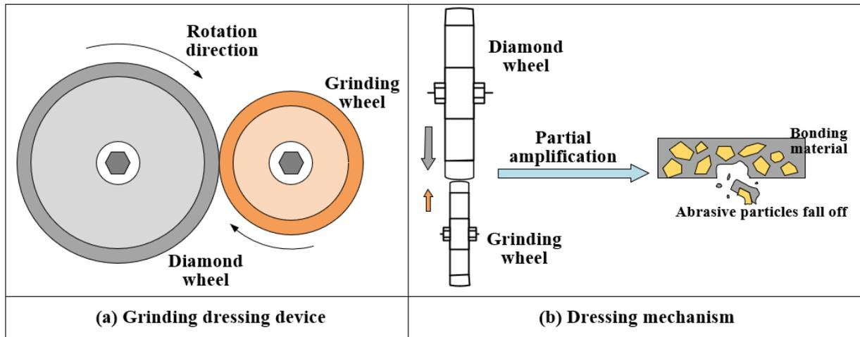
Figure 6. Schematic diagram of grinding method dressing.
