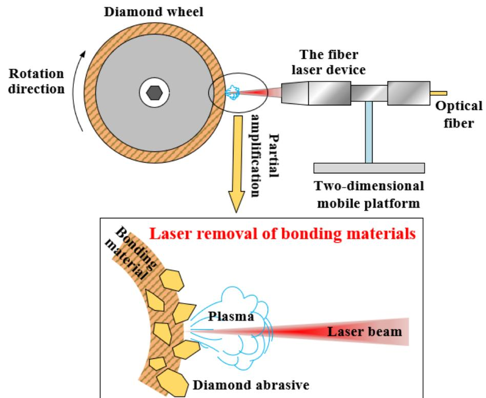
Figure 14. Schematic diagram of laser dressing diamond abrasive grinding wheel.
