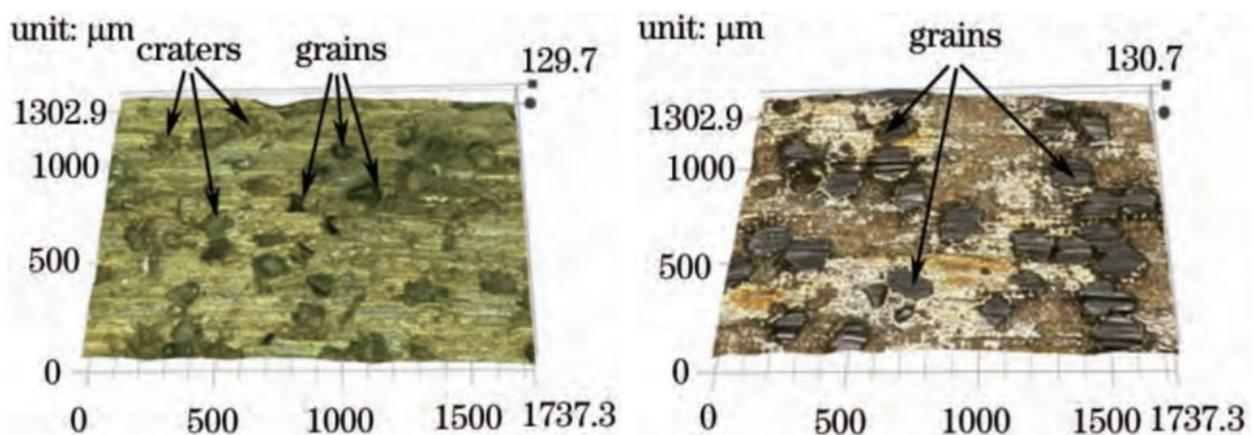
**Figure 9.** The micro-topography of the grinding wheel surface before and after laser dressing [30].
