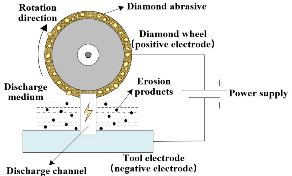
Figure 11. Schematic diagram of electric spark dressing technology.
