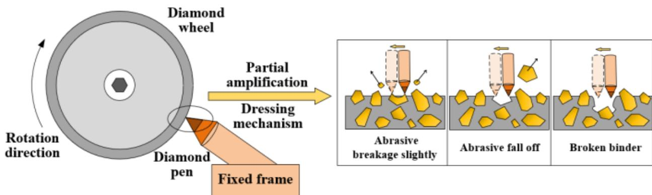
Figure 2. Schematic diagram of diamond pen dressing diamond abrasive grinding wheel.
