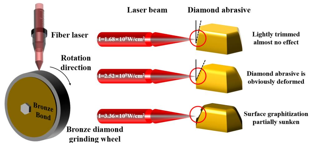
**Figure 17.** Laser dressing the bronze-bonded diamond abrasive grinding wheel experimental equipment.
