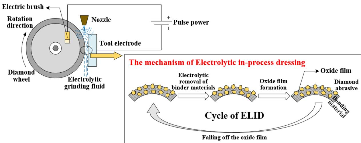
Figure 12. Schematic diagram of electrolytic in-process dressing technology.
