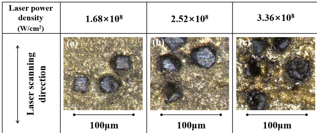
**Figure 18.** Topography of the bronze-bonded diamond abrasive grinding wheel after pulsed fiber laser dressing. (a) Laser power density:  $1.68 \times 10^8 \text{ W/cm}^2$ ; (b) Laser power density:  $2.52 \times 10^8 \text{ W/cm}^2$ ; (c) Laser power density:  $3.36 \times 10^8 \text{ W/cm}^2$ .
