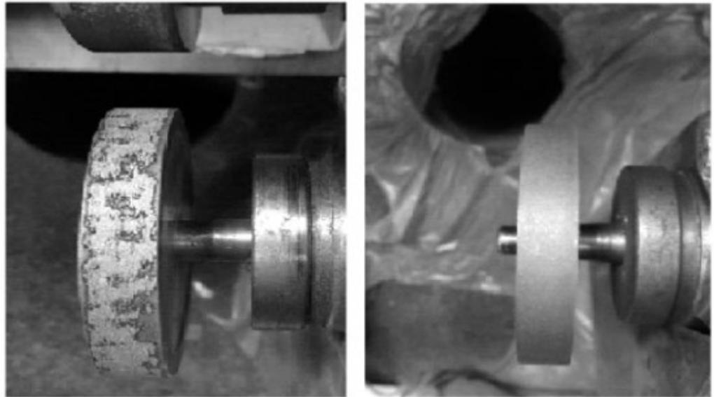
**Figure 13.** The surface condition of the grinding wheel after electric machining [44].
