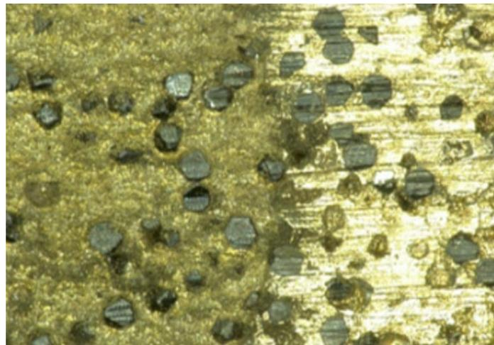
Figure 15. Topography and landform of bronze diamond abrasive grinding wheel after multi-pulse fiber laser dressing.
