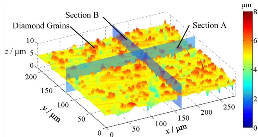
**Figure 5.** The micro-morphology of the surface of the diamond abrasive grinding wheel after dressing [11].
