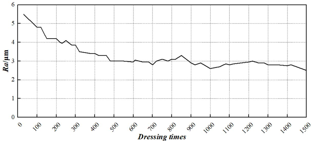
Figure 3. Variation law of grinding surface roughness Ra with the dressing times [6].
