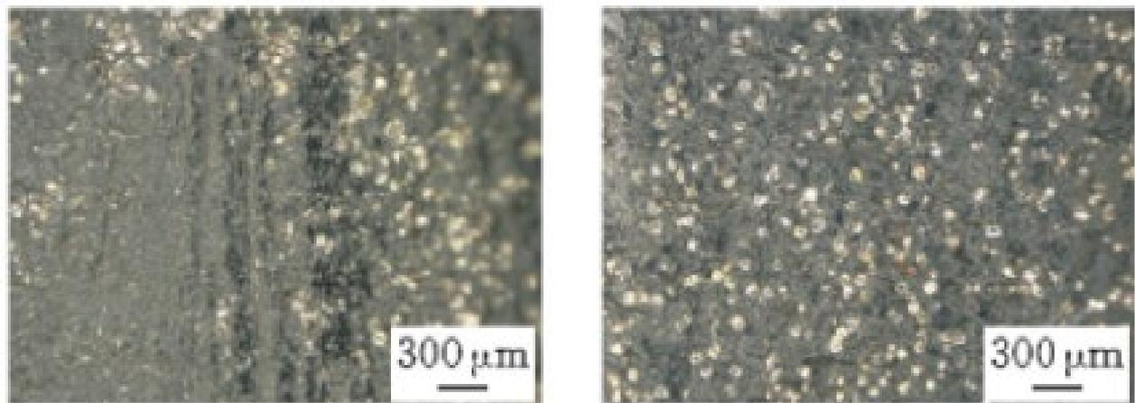
**Figure 10.** Comparison of grinding wheel surface morphology before and after grinding wheel dressing [34].
