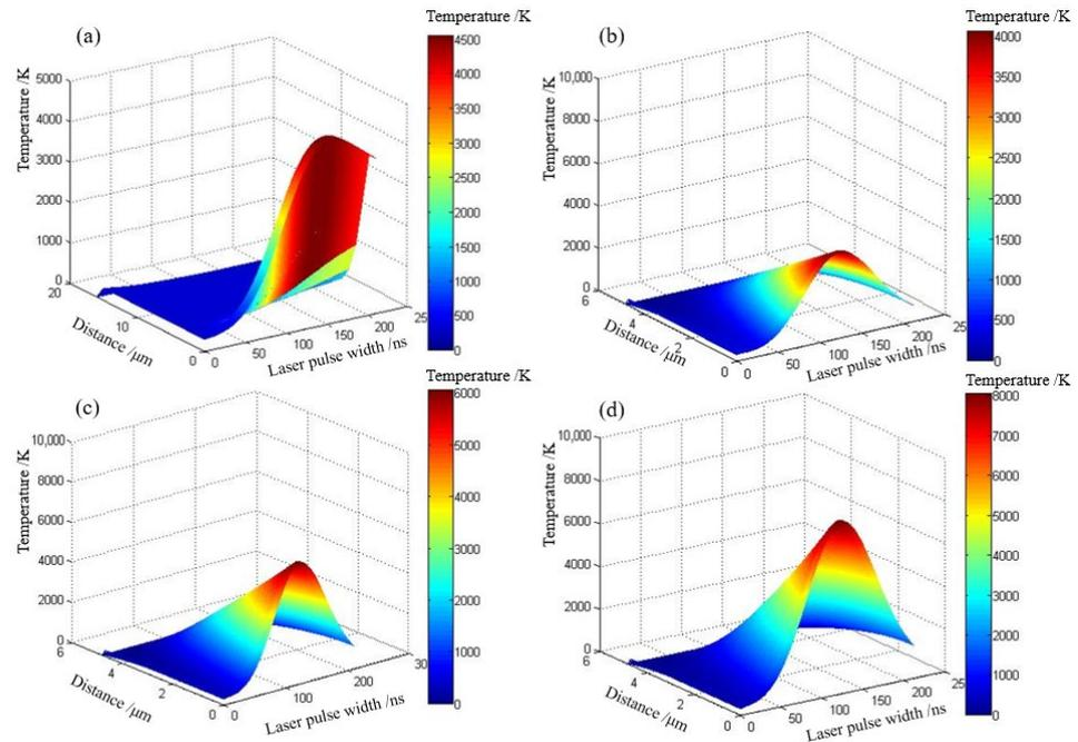
**Figure 16.** Temperature changes in the pulsed fiber laser dressing bronze material and diamond. (a) Bronze material, laser power density:  $1.68 \times 10^8 \text{ W/cm}^2$ ; (b) Diamond, laser power density:  $1.68 \times 10^8 \text{ W/cm}^2$ ; (c) Diamond, laser power density:  $2.52 \times 10^8 \text{ W/cm}^2$ ; (d) Diamond, laser power density:  $3.36 \times 10^8 \text{ W/cm}^2$ .
