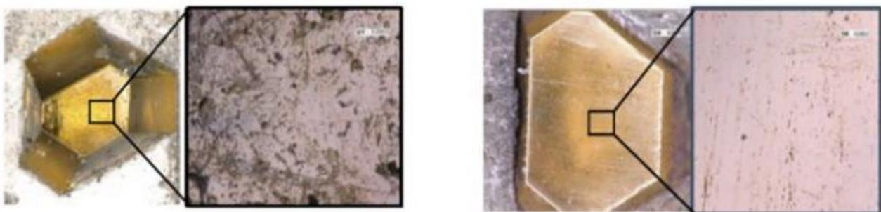
Figure 7. Surface condition before and after diamond abrasive grinding [17].
