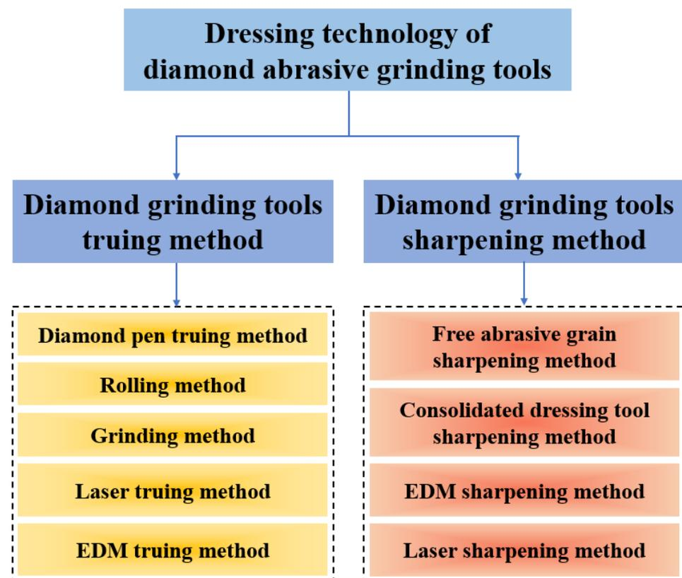
Figure 1. Diamond abrasive grinding tools dressing technology.
