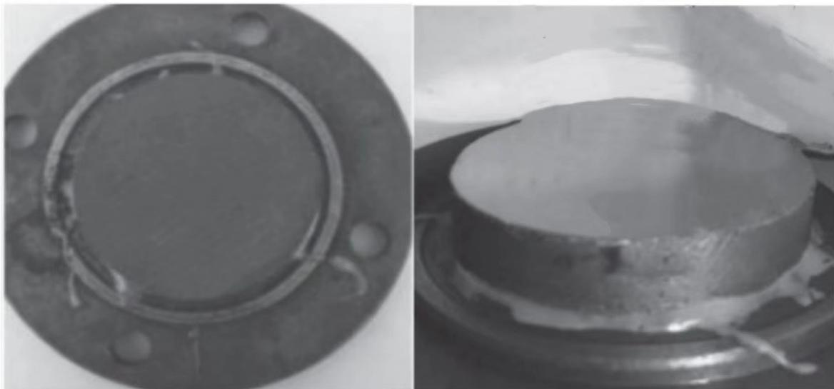
**Figure 8.** Surface renderings of the aluminum-based diamond before and after Electrolytic in-process dressing technology (ELID) processing [24].
