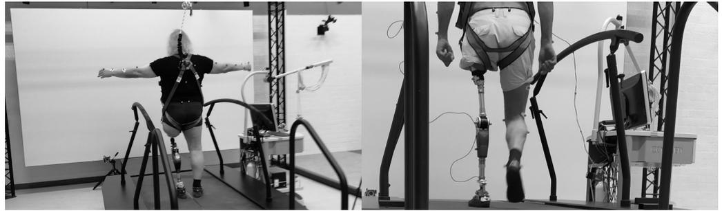
**Figure 5.** Treadmill test: the participant's movements are measured thanks to the reflective markers placed on their skin. The participant wore a harness for safety.
