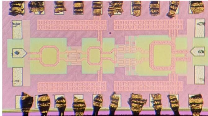
Figure 10. Photograph of the designed CMOS power amplifier ( $0.725 \times 0.55 \text{ mm}^2$ ).
