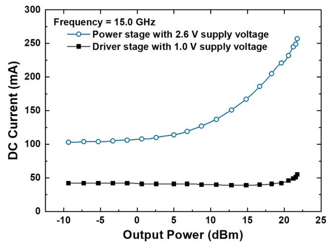
Figure 13. Measurement results: current consumptions of driver and power stages.
