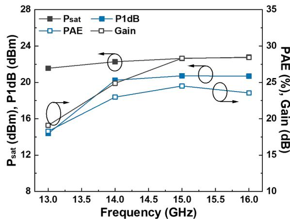
Figure 9. Simulation results:  $P_{\text{sat}}$ , P1dB, PAE, and gain depending on frequency.
