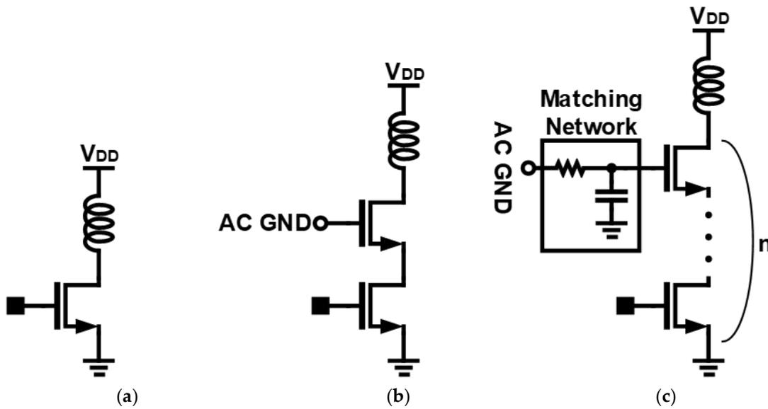
Figure 1. Typical structure of power amplifiers: (a) common-source, (b) cascode, and (c) stack structures.
