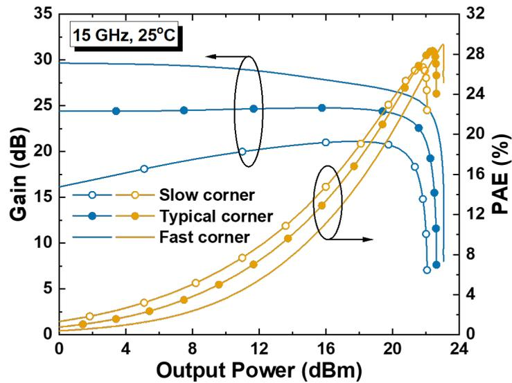
Figure 6. Simulation results: gain and PAE according to output power in slow, typical, and fast corners.
