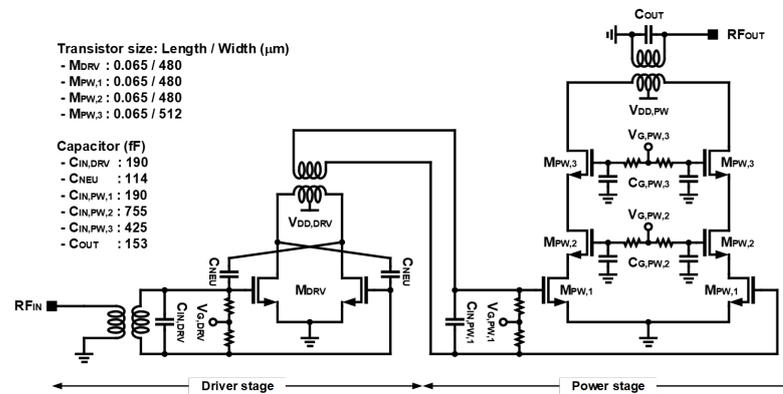
Figure 3. Schematic of designed power amplifier.
