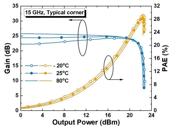
Figure 7. Simulation results: gain and PAE according to output power at operating temperatures -20 °C, 25 °C, and 80 °C.
