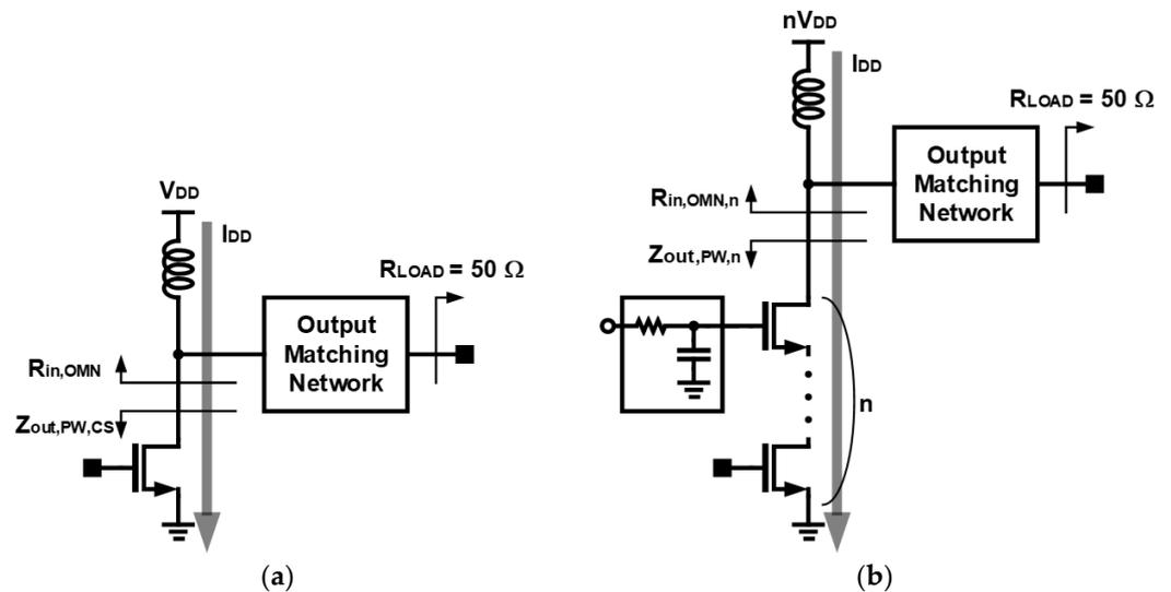
Figure 2. Impedances of power stages: (a) common-source and (b) stack structures.
