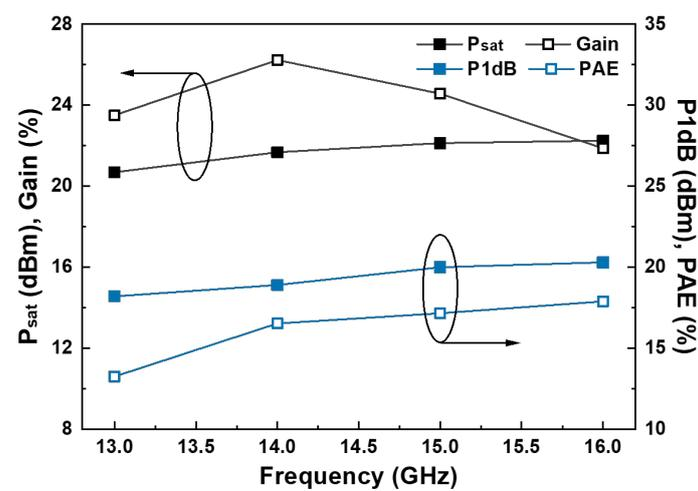
Figure 14. Measurement results:  $P_{sat}$ , P1dB, PAE, and gain depending on frequency.
