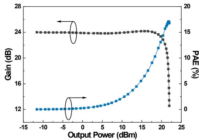
Figure 12. Measurement results: gain and PAE according to output power.
