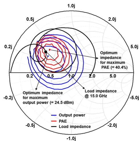
Figure 4. Load-pull simulation results.
