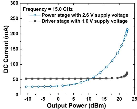
Figure 8. Simulation results: current consumptions of driver and power stages.
