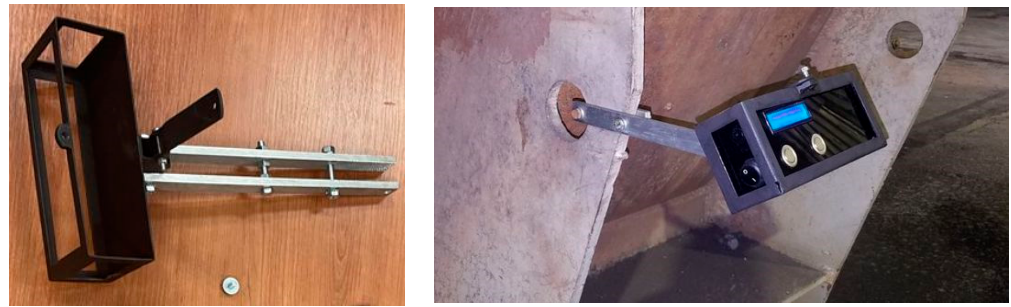
Figure 9. Installation of acquisition device: bracket for device accommodation ( left ); device mounted on the industrial coal mill ( right ).
