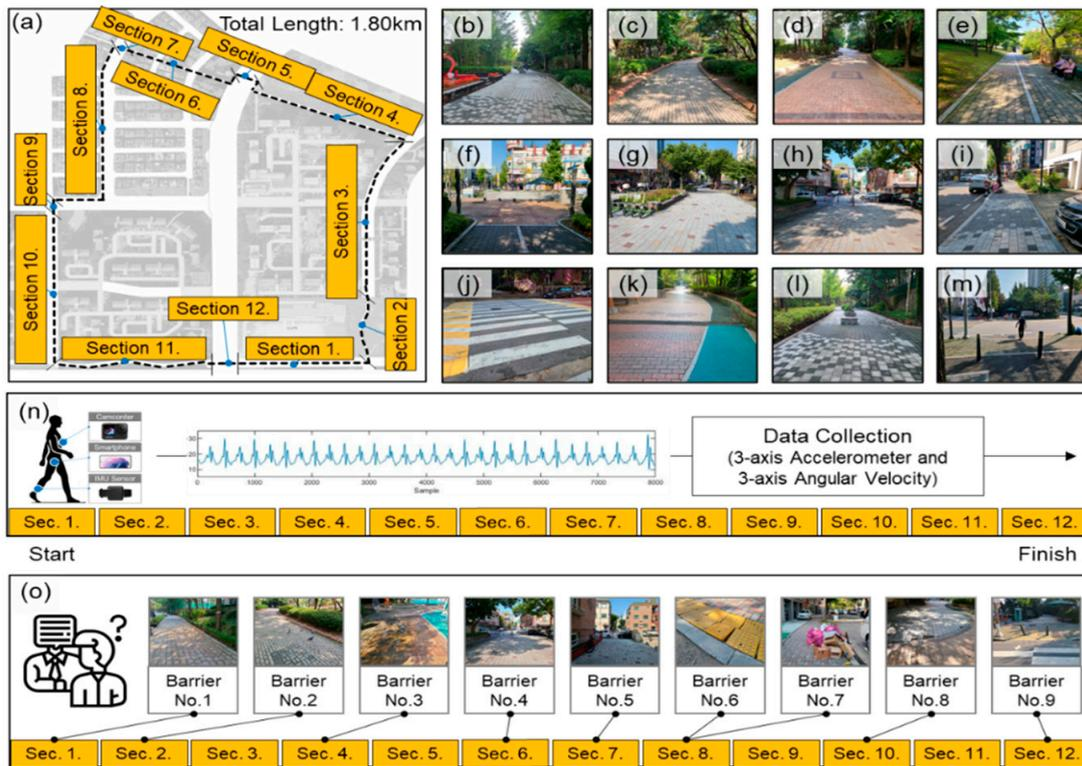
**Figure 3.** Graphical summary of experimental site and procedure; (a) site and sections; (b–m) representative pictures of each section; (n) first stage of experiment (data collection); and (o) second stage of experiment (examination and record of environmental barrier expressed by participants).
