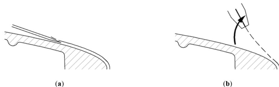
**Figure 10.** Scheme of tearing off the shield during preliminary tests: (a) crack initiation with a chisel, (b) tearing off the shield with universal pliers.
