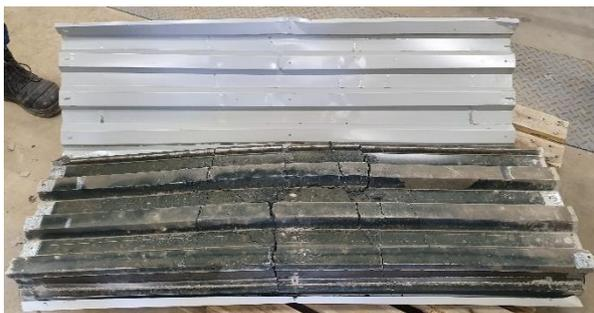
**(a)** Opened sample—Flexure cracks on the bottom surface
