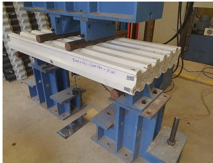
(b) Test arrangement of single-cell panel
