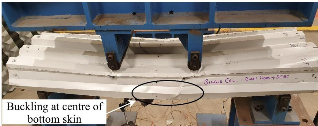
Figure 10. Compression in bottom skin due to buckling.
