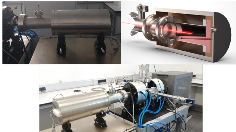
**Figure 7.** LINAC 7 beam stop (Faraday cup). Installed beam stop at the end of the LEBT for initial testing under low energy. Top right shows a cross-section of the cad model; the slanted impact face is visible there.
