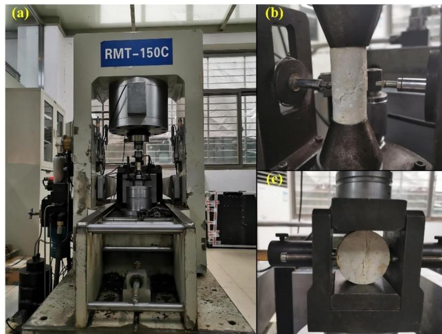
**Figure 6.** (a) The RMT multifunctional rock rigidity testing machine, (b) the uniaxial compression test, (c) the split tensile test.
