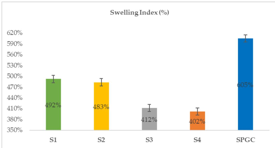
**Figure 5.** The outcomes of the nZnO particles on the starch-based films' (S1–S4) swelling index compared to the SPGC sample without nZnO.
