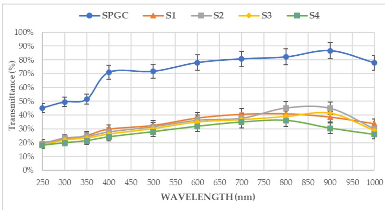
**Figure 4.** UV-Vis transmittance percentage of biodegradable starch/polyvinyl alcohol wound dressings before (SPGC) and after adding four different amounts of nano-sized ZnO particles to the material (S1–S4).
