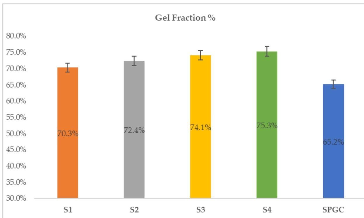
**Figure 7.** Comparison of the starch-based film (SPGC) and the samples (S1–S4) with nZnO gel fraction percentage.
