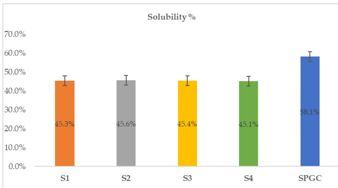
**Figure 6.** The solubility percentage of the starch-based films (S1–S4) was affected by adding the nZnO particles.
