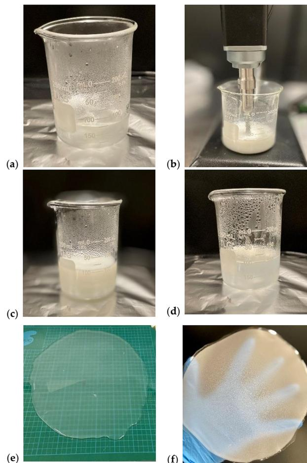
**Figure 1.** The blend-preparation steps: (a) dissolving PVA in DI water, (b) mixing starch and nZnO powder, (c) adding starch/nZnO and PVA solutions, (d) after adding glycerol and citric acid at the interval of 10 min, (e) pouring the final solution on the flat glass, (f) starch-based polyvinyl alcohol (PVA) blend with inserted nano-zinc-oxide particles (nZnO).
