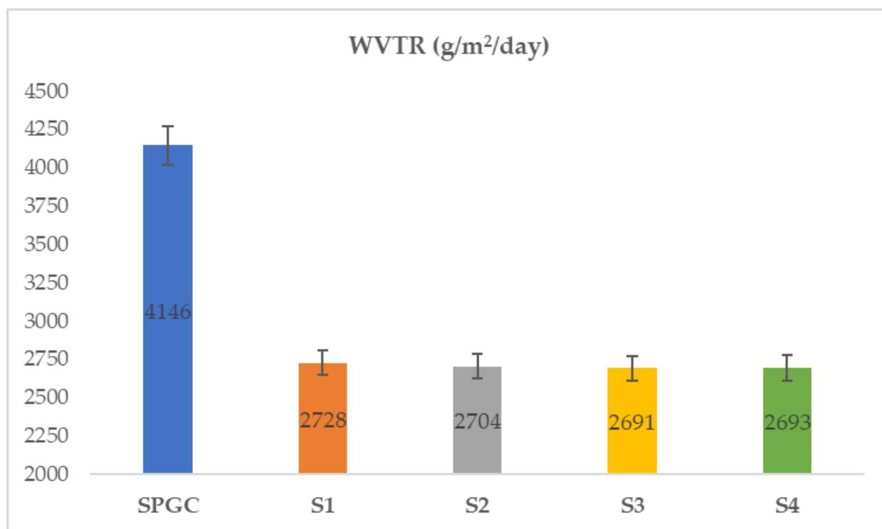
**Figure 3.** Biodegradable starch/PVA wound dressings' WVTR before (SPGC) and after adding nano-ZnO particles (S1–S4) to the starch-based/polyvinyl alcohol composite.
