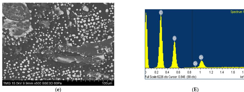
**Figure 11.** EDX spectra (A–E) and SEM images of (a) starch/polyvinyl alcohol/citric acid/glycerol (SPGC), and starch/polyvinyl alcohol/citric acid/glycerol/nZnO films, (b) 0.2 g nZnO (S1), (c) 0.25 g nZnO (S2), (d) 0.3 g nZnO (S3), (e) 0.35 g nZnO (S4).
