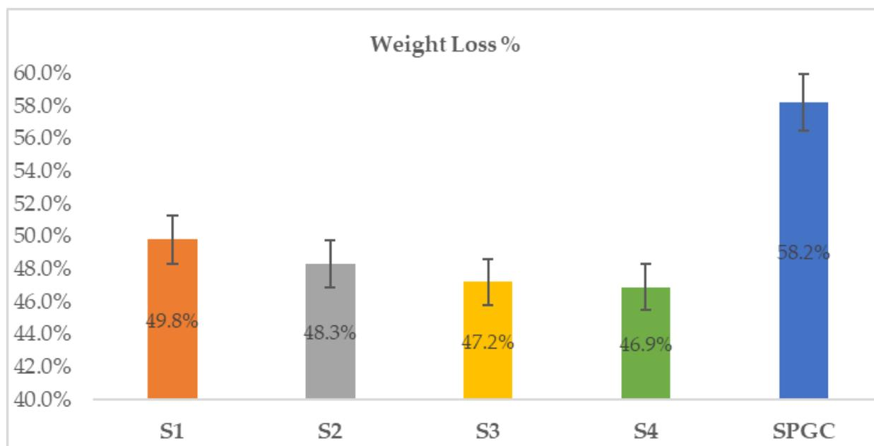
**Figure 8.** Weight-loss percentage comparison of the starch-based film (SPGC) and the samples (S1–S4) with nZnO.
