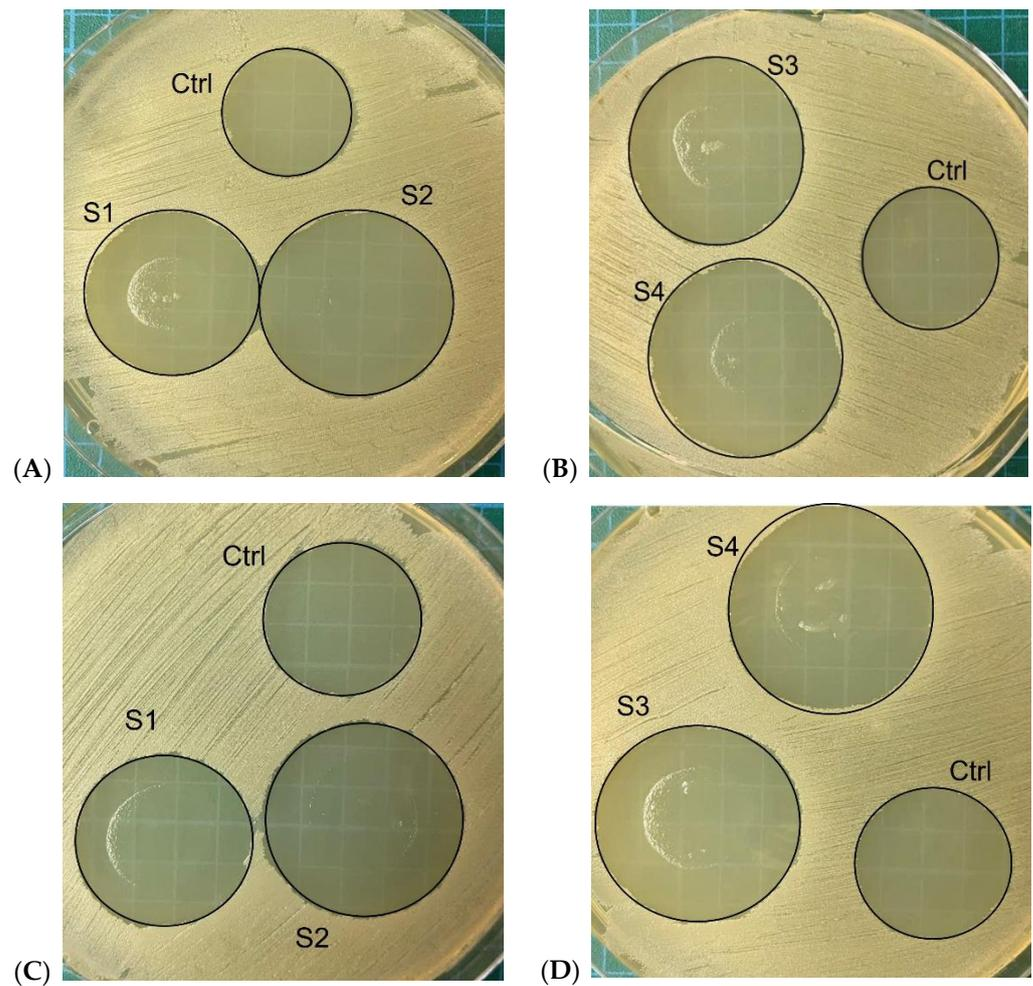
**Figure 12.** Antibacterial activity test of starch-based materials against *E. coli* and *S. aureus* in formulations with different weight ratios of ZnO nanoparticles: (A,B) images of S1–S4 samples tested against *E. coli* and their control zones using Penicillin; (C,D) images of S1–S4 samples tested against *S. aureus* and their control zones using Penicillin.
