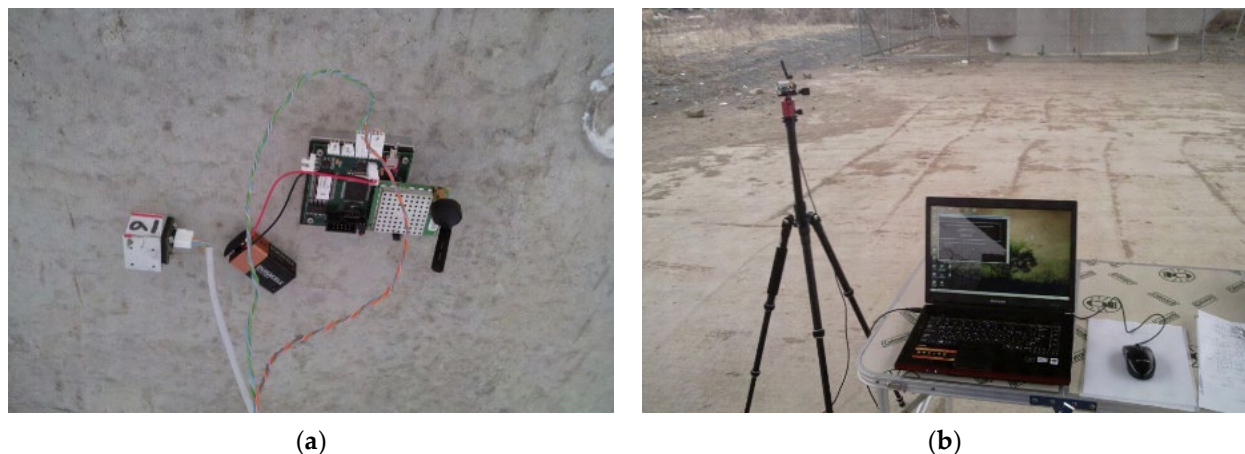
Figure 2. Wireless measurement system: (a) NARADA WSU and accelerometer; (b) Base station and laptop.
