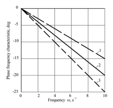
**Figure 5.** Phase-frequency characteristic of the tractor course angle  $\varphi$  when working out perturbations by it in the form of oscillations of the haulm harvester's steering angle  $\beta$  at different unit movement speeds:  $1-V_0 = 1.5 \text{ m}\cdot\text{s}-1$ ;  $2-V_0 = 2.0 \text{ m}\cdot\text{s}-1$ ;  $3-V_0 = 2.5 \text{ m}\cdot\text{s}-1$ .
