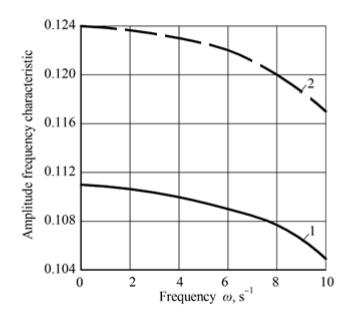
**Figure 6.** Amplitude-frequency characteristic of the course angle  $\varphi$  of the tractor when it works out disturbances in the form of oscillations of the angle  $\beta$  of rotation of the harvester at different values of the input resistance coefficient  $k_A$  of pneumatic tires of its front steerable wheels: 1–120 kN·rad<sup>-1</sup>; 2–80 kN·rad<sup>-1</sup>.
