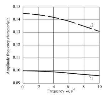
**Figure 7.** Amplitude-frequency characteristic of the tractor course angle  $\varphi$  when working out disturbances in the form of oscillations of the harvester machine rotation angle  $\beta$  at different values of the input resistance coefficient  $k_B$  of pneumatic tires of rear traction wheels: 1–150 kN·rad<sup>-1</sup>; 2–90 kN·rad<sup>-1</sup>.
