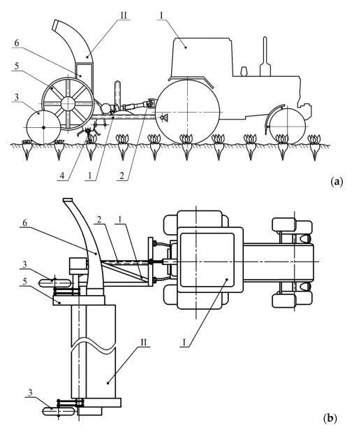
**Figure 1.** Construction and technological scheme of asymmetric of the haulm harvester (**a**)—side view; (**b**)—top view: I—wheeled tractor; II—trailed asymmetric haulm harvester: 1—frame; 2—drive; 3—support-copying pneumatic wheel; 4—rotary haulm cropper; 5—transporting working device; 6—loading device.
