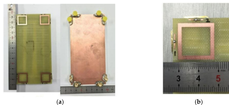
Figure 6. MIMO antenna with orthogonal polarization: (a) geometry of proposed MIMO; and (b) antenna element with dual-polarized modes (Results from [61]).
