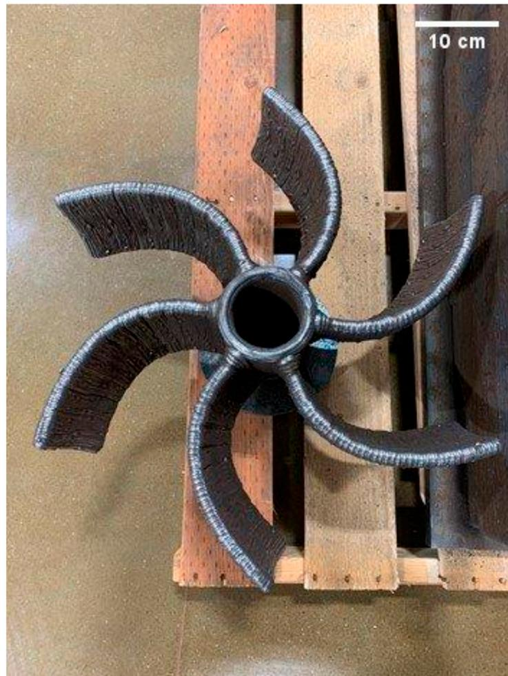
**Figure 1.** Wire arc manufactured propeller demonstrator at Oak Ridge National Lab Manufacturing Demonstration Facility. The propeller was printed in 20 h and weighed around 60 kg.
