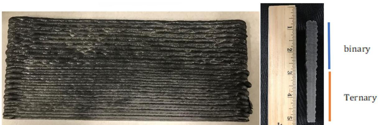
**Figure 8.** Side and cross-sectional views of wall deposited by altering the shielding gas from ternary blend to binary blend midway through the build.
