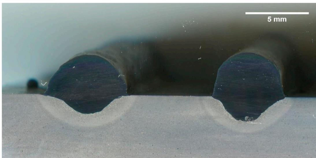
**Figure 6.** Bead-on-plate experiment using a binary (left) and ternary blend (right).
