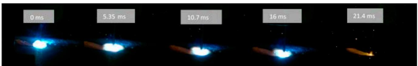
**Figure 2.** The arc appearance, labeled with the timing from the droplet initiation to detachment, for the ternary blend.
